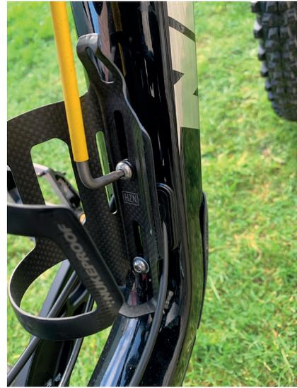
4. Slide the cage to the desired position and tighten bolts. Your Nukeproof cage has 40mm of adjustment.
