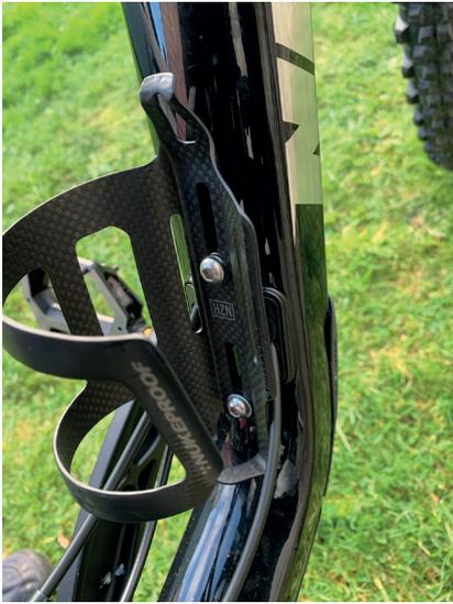
3. Put the bottle cage on your frame and insert both bolts.
