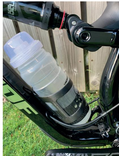
6. On a full suspension frame, it can be worth "bottoming out" the shock to ensure that the cage or bottle is not in the way as the frame goes through its travel.
