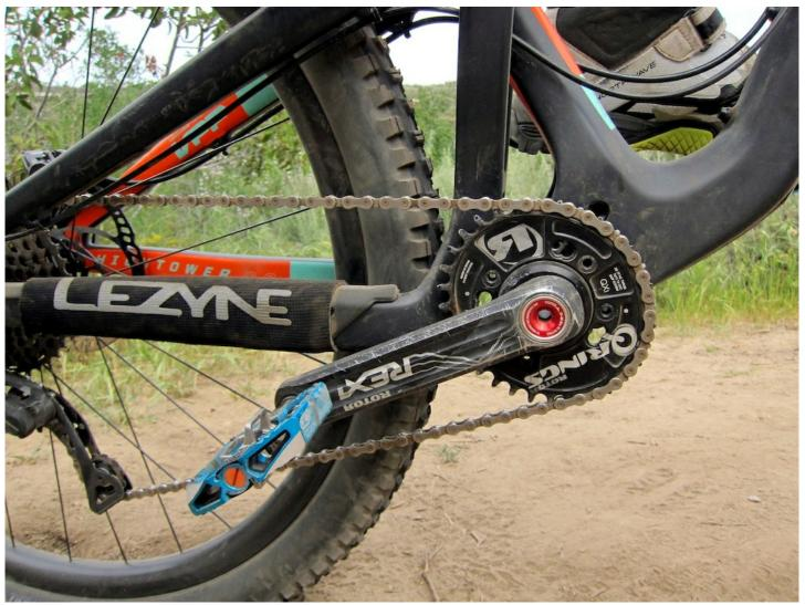
Cracia runs a Rotor Rex 1 aluminum crankset and a QX 1 chainring. Three mounting positions on the chainring are used to time the rider's power-stroke with his or her riding position over the crankset, and to compensate for variations in leg kinematics.
