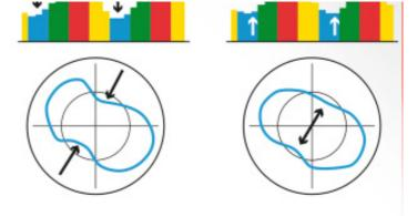
Rotor has done extensive comparative testing to verify the attributes of ovalized chainrings. Torque measured at the crank axle shows that the round chainring (left) produces a more erratic pedaling stroke, while the oval Q-Ring (right) produces more consistent torque throughout the pedal circle (I did this comparison test and it produced similar results - RC).
