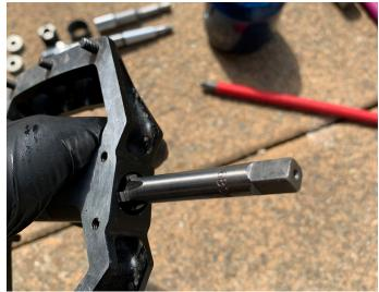
6. Use the tap from the Nukeproof Bushing Removal tool kit to insert into the bushing and turn. The first couple of turns will be tough then you will feel the bushing start to spin in the pedal body. At this stage pull the tap out of the pedal and the bushing will come with it.
