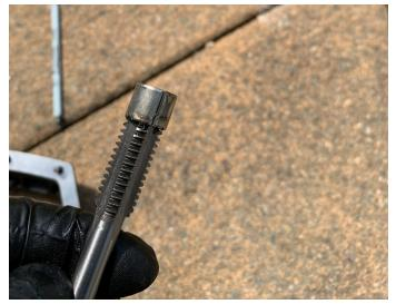
7. The bushing has a split design so you can use your flat head screwdriver to prize it open and remove it from the tap.
