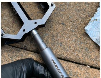
10. Get the bushing install tool, put the bushing on the end of the tool and push it into the pedal body. A firm press is required to ensure it is fully inserted.
