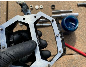
8. Clean the inside of the pedal body with paper towel. This can be pushed through the body with a hex key or an old spoke.
