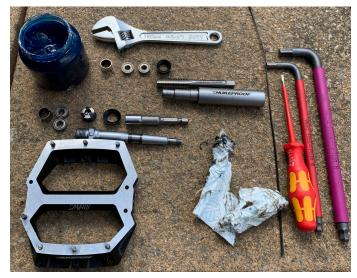
9. The pedal has now been stripped. Discard any old parts so they do not get mixed with new parts.
