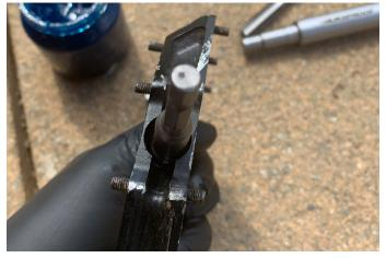
13. Push bearings into place using the pedal nut socket and then retighten nut.
