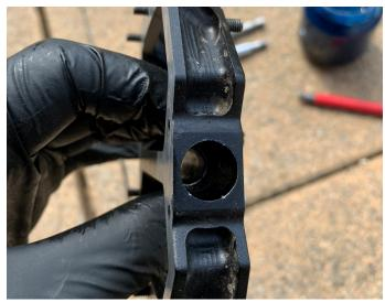
5. Visually locate the bushing in the pedal body, it will be visible from the inner side of the pedal body.
