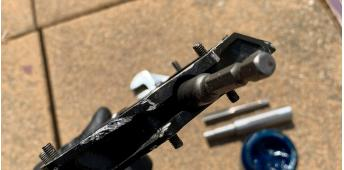
Insert your 8mm into the pedal axle and use the nut socket remover to remove the nut from the axle.
