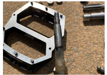
3. Remove the axle from the pedal, remove the seal from the pedal and clean parts with paper towel.
