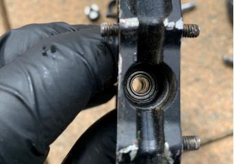
4. Using your 1.5mm or 2mm hex key, remove the bearings from the pedal by hooking with the L shape of the hex key.
