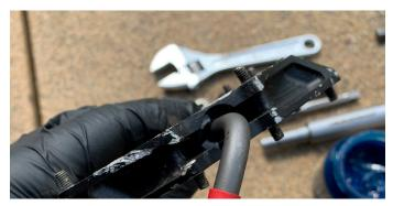
1. Using your 6mm hex key, remove the end cap from the pedal.
