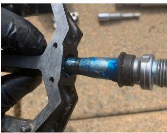
11. Take your axle, install the new seal, apply grease and insert into pedal body.
