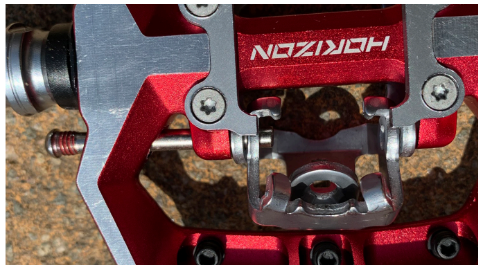
20. Fit the other part of the binding and push the pin further through to hold it in place.
