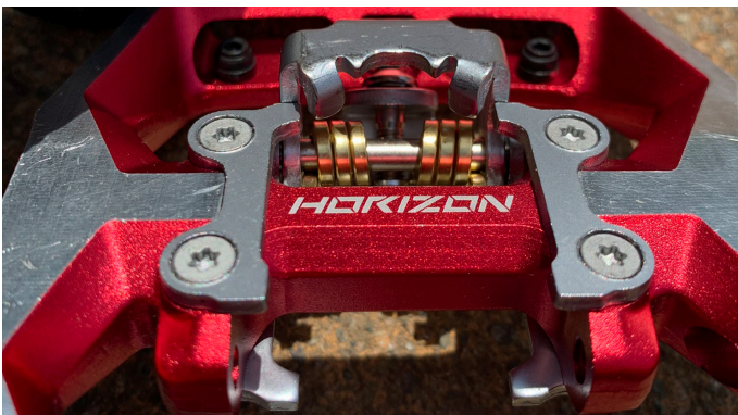
21. Get your springs and look at the direction of the coils to determine which order they need installed in. When they are installed the coils will point in opposite directions.
