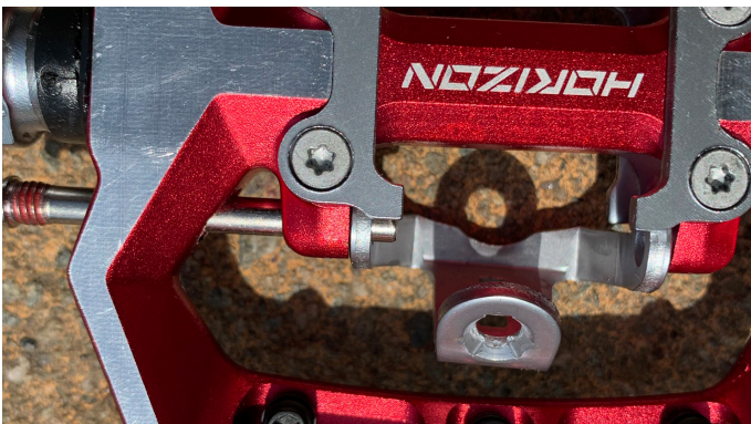
19. Get one binding set and install the into the pin and the first part of the binding with the tension adjuster screw hole into the pedal body.
