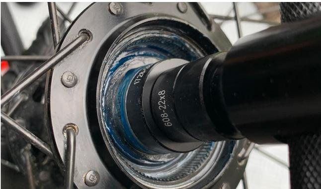
3. Press the bearing into the shell. Ensure it spins smoothly.
