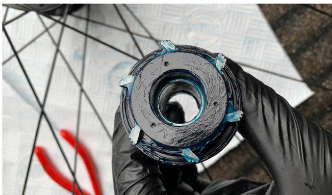
3. Apply a layer of grease to the rear of the freehub over the pawls and springs.
