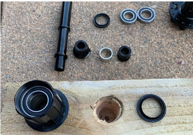
9. Get your freehub and remove seal from outside bearing using a flat head screwdriver.
