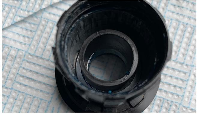
2. Get the spacer and set into the freehub. This should sit central on the bearing you pressed in.
