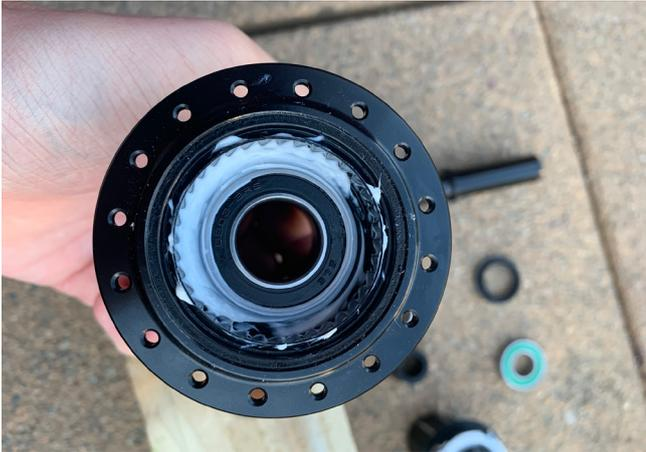
7. When the bearing has been removed from the non-driveside, the axle will pull out of the hub so it can now be removed.
