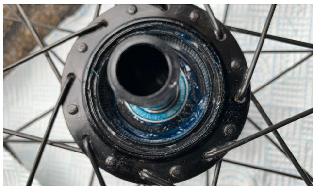
2. Apply a layer of grease to the ratchet ring and around the driveside bearing in the hub shell.
