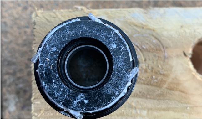
13. Using your bearing punch, hit the last bearing out of the freehub. Again, this bearing should be hit in various places to ensure it comes out straight.
