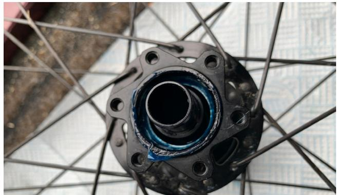
4. Put the axle into the hub through the non-driveside.
