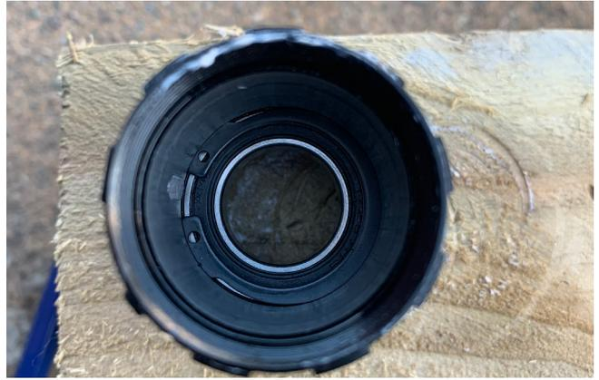
12. The last bearing is held in place by a circlip, use internal circlip pliers with 1.3mm tips to get the circlip out.
