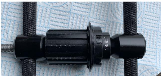
3. Get your press and correct drift, press the bearing into the freehub.
