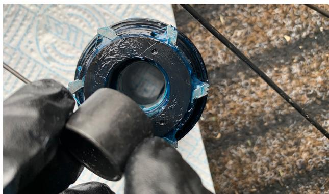
4. Refit the freehub spacer into the rear of the freehub.
