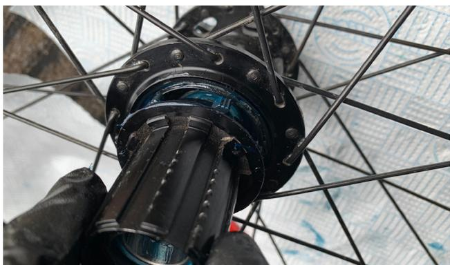
5. Slot the freehub over the axle, push onto the hub turning **ANTICLOCKWISE** as you do this to prevent damage to the seal.
