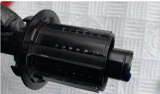
5. With the bearings now in place, take your axle and push it through the freehub to ensure the spacer is now fully central and the axle goes through correctly.
