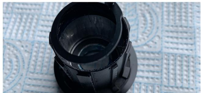
4. Get the circlip and install Infront of the bearing.
