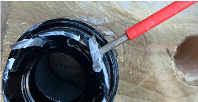
15. Remove the pawls using the flat head screwdriver.
