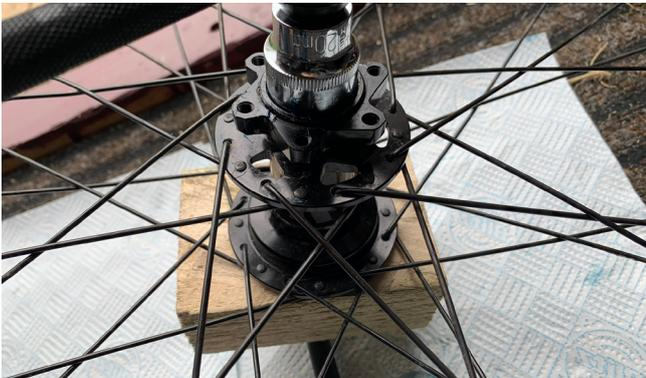
5. Take your non-driveside bearing and press it into place. On this we have used the block of wood to allow the axle to "float" and for the press to then push against the hub shell to allow the non-driveside bearing to be pushed into place.
