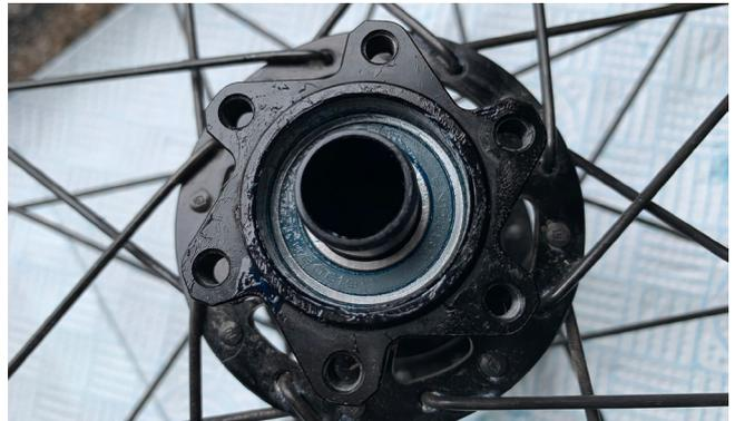
6. Apply a layer of grease to the non-driveside bearing.
