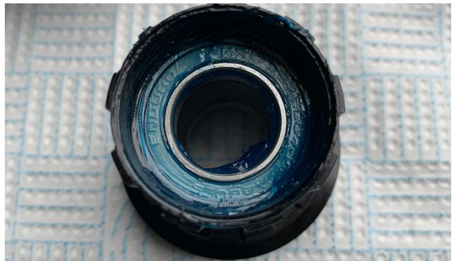
6. Apply grease on the outside of the bearing.
