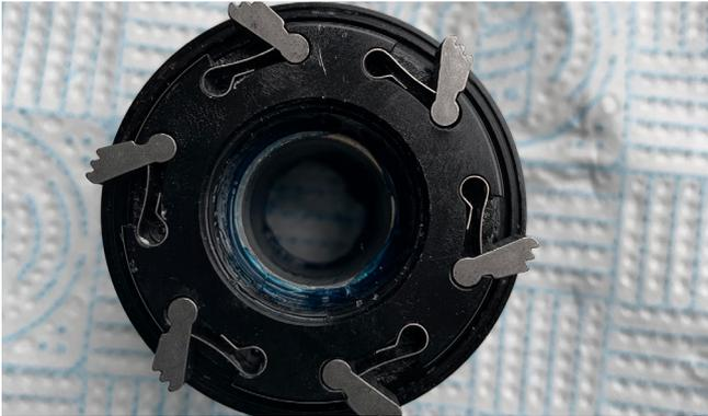
3. Check pawls and springs are fitted the correct way round and function correctly by pressing them.
