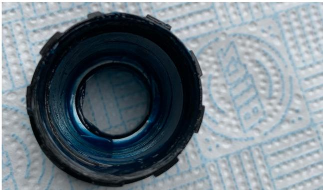
1. Check the internal of the freehub is smooth and free from burrs then apply a layer of grease inside – this is to aid the bearing installation.
