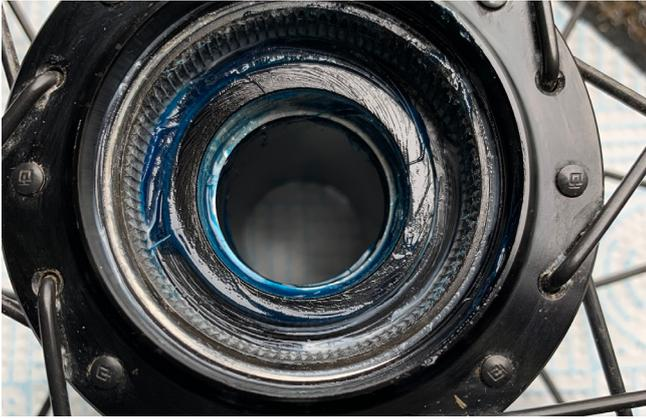
1. Check both sizes of the shell where your bearings will be pressed are smooth and free from burrs then apply a layer of grease.
