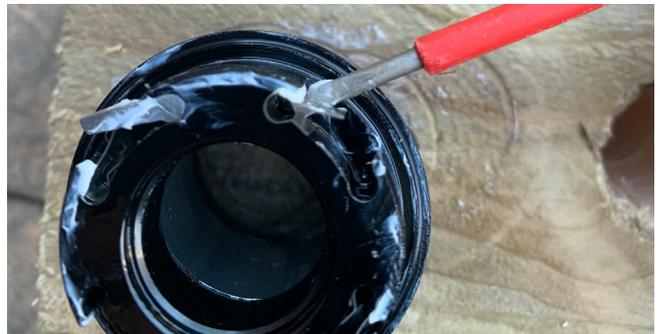
16. Remove the springs using the flat head screwdriver.
