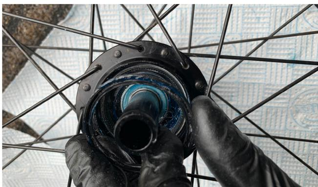
1. Apply a layer of grease to the hub shell freehub seal and push onto hub shell.
