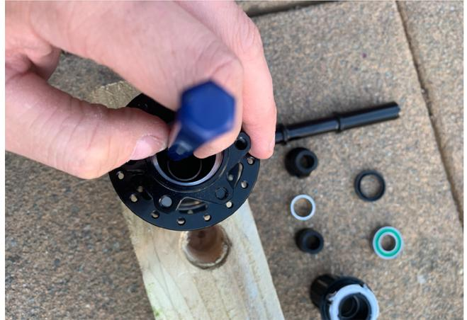
8. Turn the hub over so it is now driveside down. Using a bearing punch, hit the driveside bearing out from the back. After each hit, move position on the bearing for the next hit so it comes out evenly.
