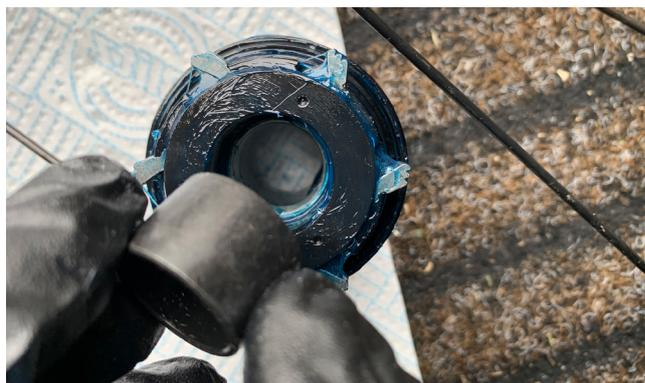
4. Refit the freehub spacer into the rear of the freehub.
