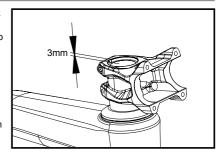
Re-install the two steerer clamp bolts, ensure stem is straight then tighten bolts to 6Nm torque.
