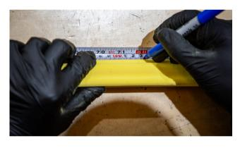
3. LAY THE ARD OUT FLAT AGAINST THE TAPE MEASURE AND MARK IT AT THE DESIRED LENGTH FOR YOUR WHEEL SIZE.
