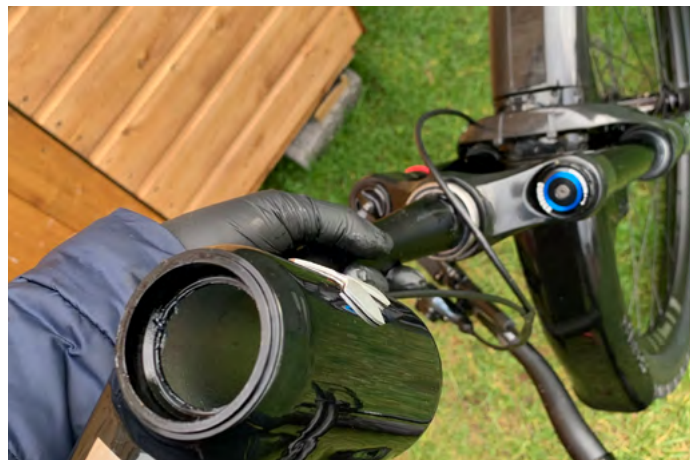
15. Put your fork back into the frame and seat bottom bearing.
