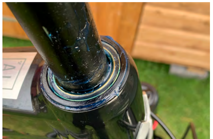
17. Apply a layer of grease around the top of the bearing.
