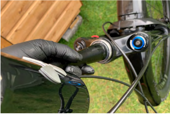
9. Carefully remove fork from the frame.
