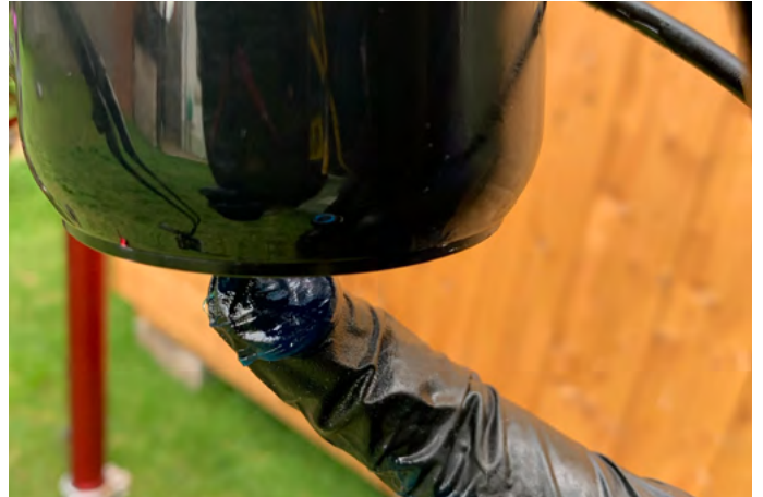
13. Apply fresh grease to lower cup.
