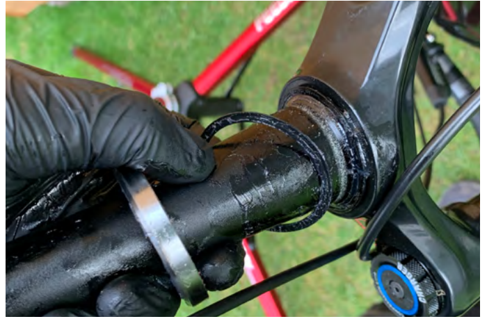
10. Remove the lower headset bearing and cover from the fork or from inside the bottom headset cup.
