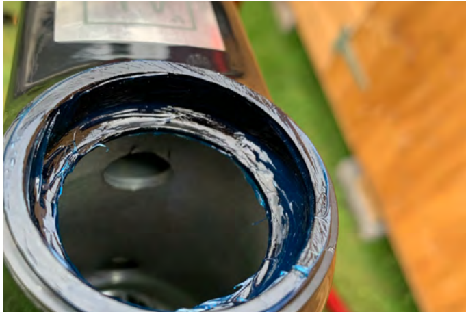
12. Apply fresh grease to the upper cup.
