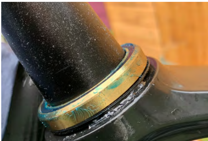
14. Get your lower headset bearing and put it onto the fork. Note: The chamfered edge should be facing upwards.
