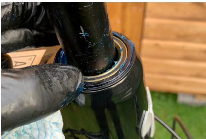
16. Refit the top bearing. Note: The chamfered edge should be downwards.
