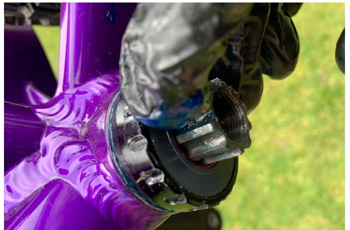
19. Apply grease to the spindle splines on the non driveside.
