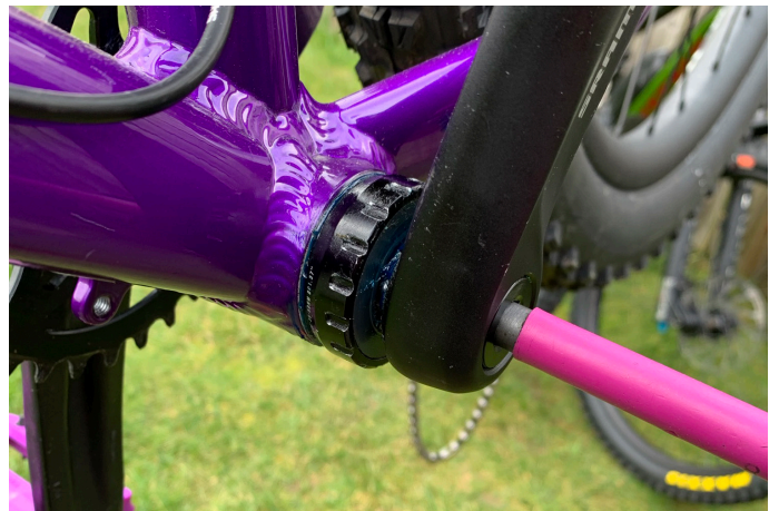
21. Tighten the crank bolt with an 8mm hex key until all play has been removed.
