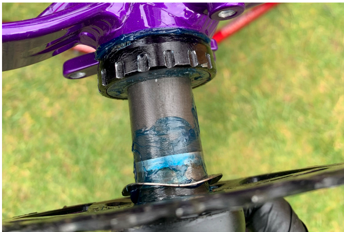
18. Fit the driveside crank by pushing the spindle through the driveside bottom bracket cup.
