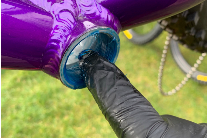
11. Grease both sides of the bottom bracket shell.
