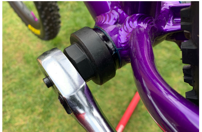
15. Take the L (non-driveside) cup, fit any required spacers. Start to install the cup into the frame by hand. The cup should turn clockwise with very little resistance. Thread locking compound has been applied to the bottom bracket threads by our factory. Tighten with a torque wrench to 35Nm – 50Nm. If there is alot of resistance when you are installing the cup - STOP . Check you have the correct cup and that it is being inserted correctly. If you are unsure consult a local bike shop.
