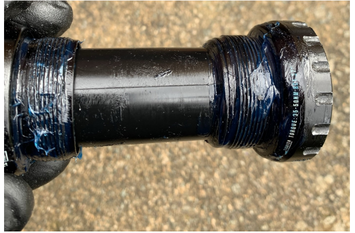
12. Grease the threads on the bottom bracket cups.
