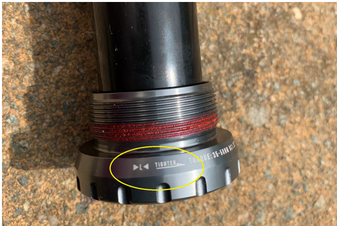
13. Check the markings on the bottom bracket cups to determine L (non driveside) and R (driveside). The cups are also etched with the direction you need to turn to tighten.
