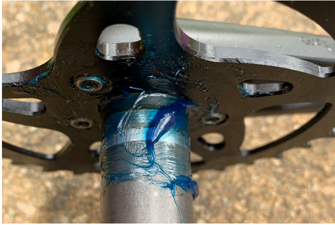
16. Apply grease to the bearing seat on the driveside crank spindle.
