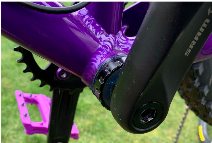
20. Fit the non drive crank arm and ensure it is 180 deg from the driveside.
