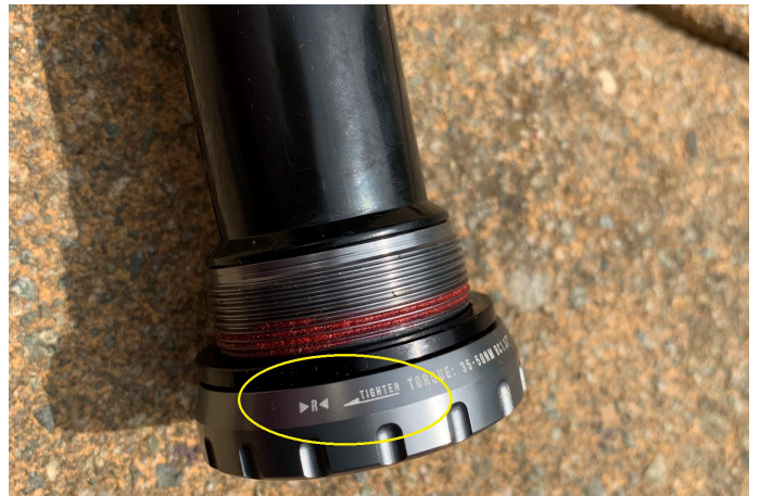
13. Check the markings on the bottom bracket cups to determine L (non driveside) and R (driveside). The cups are also etched with the direction you need to turn to tighten.
