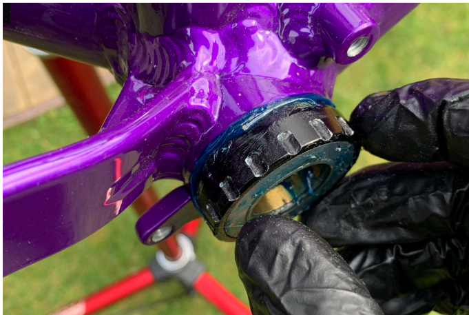
14. Get the R (driveside) cup with the centre sleeve and fit any required spacers then start to screw into the frame by hand. The cup should turn anticlockwise with very little resistance. Thread locking compound has been applied to the bottom bracket threads by our factory. Tighten with a torque wrench to 35Nm – 50Nm. If there is a lot of resistance when you are installing the cup - STOP . Check you have the correct cup and that it is being inserted correctly. If you are unsure consult a local bike shop.
