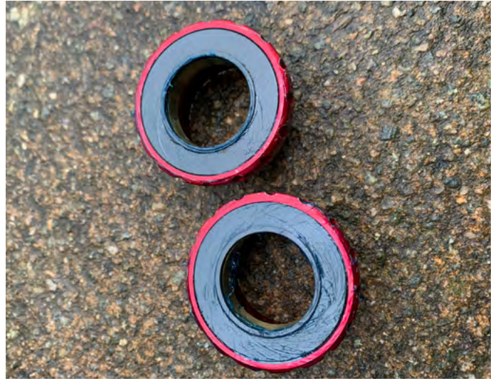
15. Your bearings are now replaced, and you can refit your bottom bracket to your frame.
