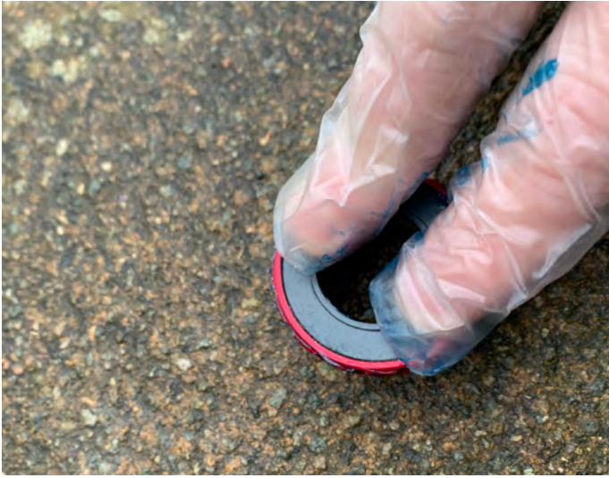
14. Press the outer seal back onto outside of the bearings.
