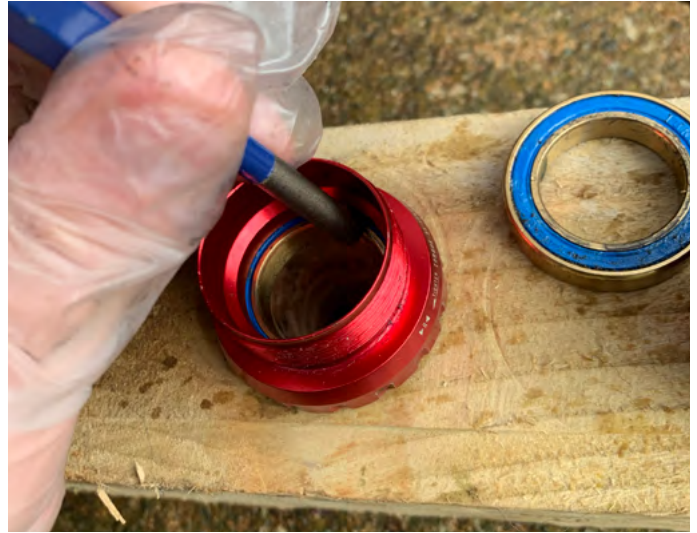
4. Take the right hand cup, place it face down on the wood, use a bearing punch to carefully knock the bearing out from the rear.
