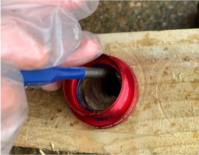
3. Take the left hand cup and place it face down on the wood, use the bearing punch to carefully knock the bearing out from the rear.
