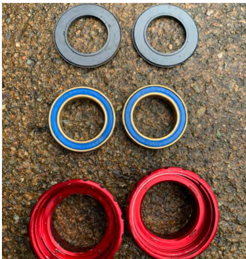
7. Your bottom bracket bearings are now disassembled.
