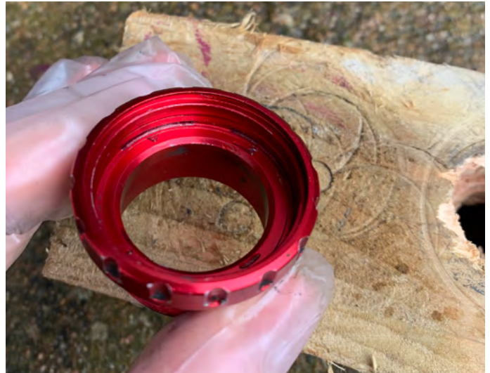
6. Inspect both cups to ensure they are free from damage.
