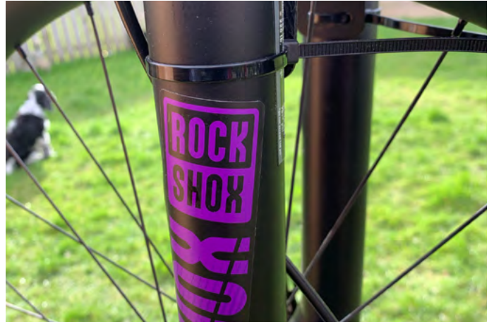
6. Rotate the cable tie so the locking mechanism is out of sight.
