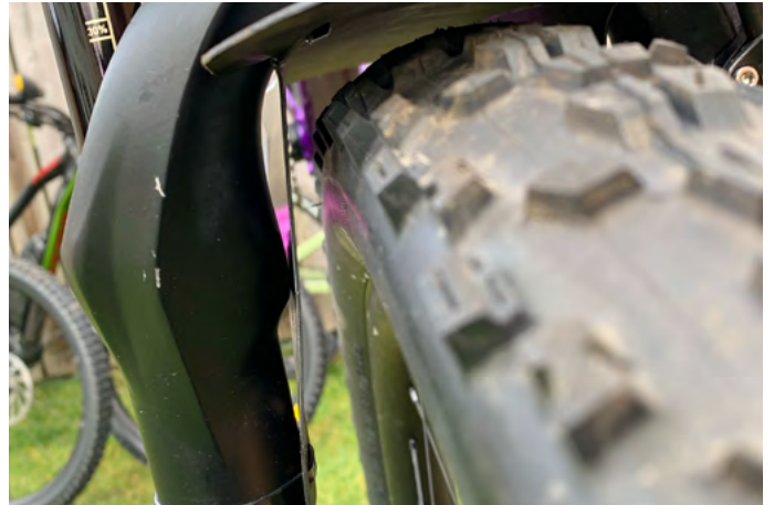
8. Check around the mudguard/tyre to ensure that the wheel is free to move with no obstruction.
