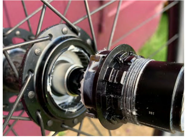
3. Pull off freehub as you turn it ANTI CLOCKWISE .
