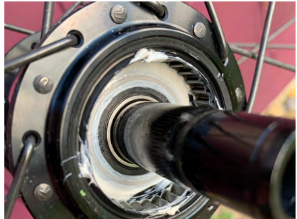
5. Inspect the hub seal for damage.
