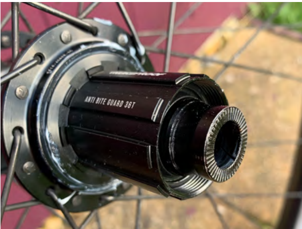
15. Push the freehub onto the hub shell turning ANTI CLOCKWISE
