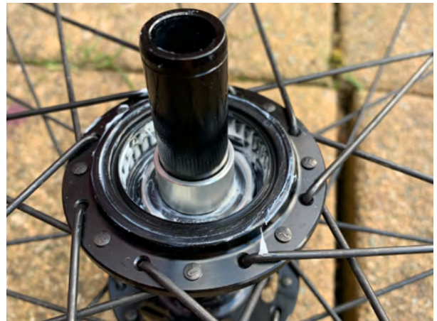
12. Push the seal into the hub shell and ensure it is correctly seated.
