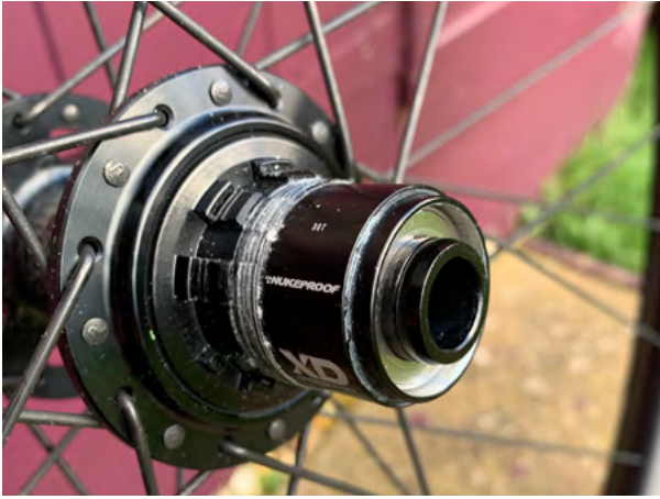
2. Remove the driveside end cap.
