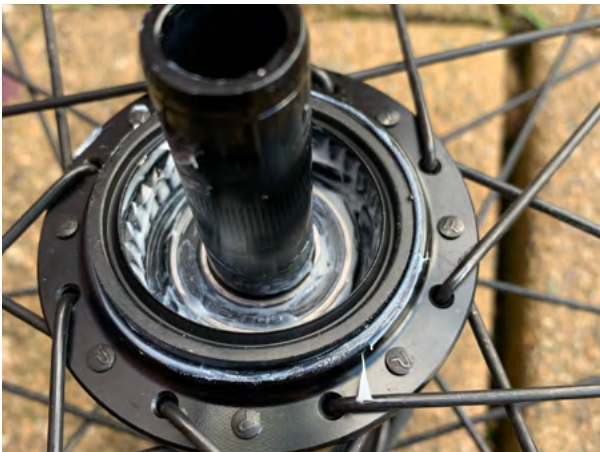
11. If you removed the hub seal in step 6, get the new seal and determine front and rear. The front of the seal has the V shape groove.
