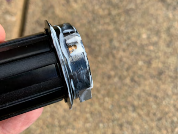
13. Refit bushing on axle.
