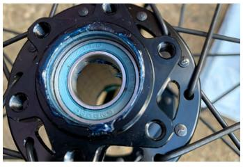
15. Continue to finish pressing the bearing so it has been 16. If the sub axle has moved slightly off centre, this can fully seated correctly.
