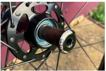
14. As the sub axle needs lined up, it is important to STOP pressing in the bearing when you start to feel resistance. At this stage get your fork thru axle and put it through the hub to line up the sub axle.
