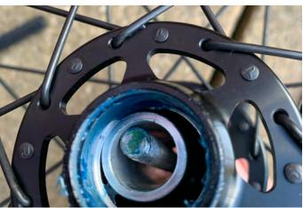
12. Put the sub axle back into the hub.
