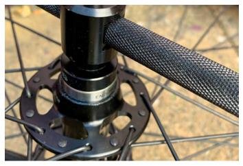
13. Carefully set the other bearing into position on the hub shell then put your bearing press through the bearing and hub. Use the correct size of bearing drift and start to press in the bearing. Note: If you are using the Nukeproof Enduro bearings, the blue seal faces outwards.
