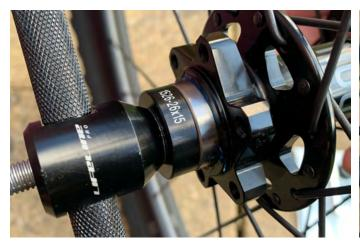
11. Carefully put your bearing press through the bearing and hub. Use the correct size of bearing drift and press in the bearing.
