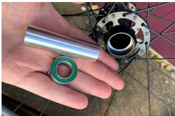
One bearing and the sub axle should now be out of the hub.
