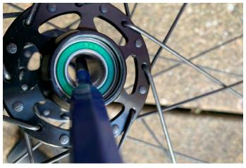
Push the sub axle which sits between the bearings off centre. If it won't move by pushing with your finger you can use a bearing punch or screwdriver to gently push it.
