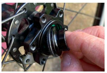
. Remove non driveside end cap by pulling it off. Pliers can be carefully used if it is stuck to assist.
