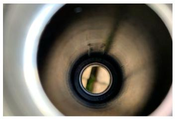
7. Repeat the process on the other bearing to remove it 8. from the hub by knocking it out from behind.
