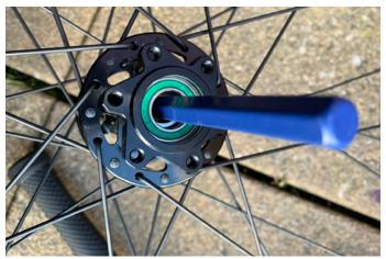
5. Use a bearing punch to carefully knock the bearing out. **Note:** You should work your way around the bearing so that it comes out evenly.
