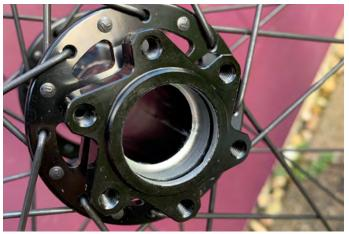
. With the bearings now removed from the hub. Check the hub shell for damage and clean.
