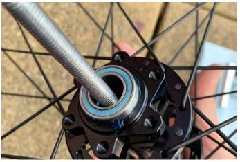
10. Get your new bearing and set it into position. **Note:** If you are using the Nukeproof Enduro bearings, the blue seal faces outwards.
