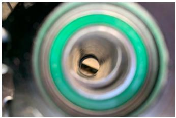
With the sub axle now off centre, check that you can see the back of the bearing by looking through the hub shell.
