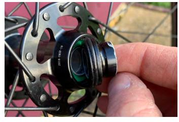
Remove driveside end cap by pulling it off. Pliers can 2. be carefully used if it is stuck to assist.
