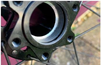
9. Apply grease to the bearing seats on both sides of the hub.
