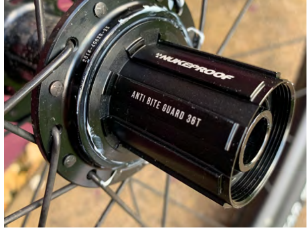
14. Push the freehub onto the hub shell turning ANTI CLOCKWISE
