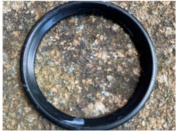
10. If you removed the hub seal in step 6, get the new seal and determine front and rear. The front of the seal has the V shape groove.
