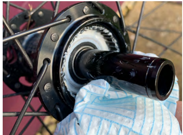
7. Clean off the old grease and ensure no other parts are worn or damaged.
