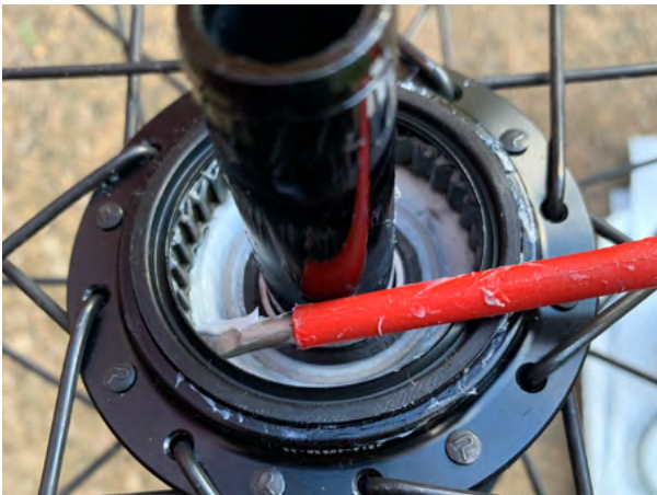
6. If the seal is damaged, remove it by pushing a flat head screwdriver or pick underneath and pull it off.
