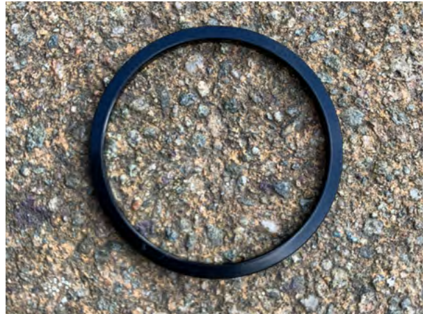
16. If you have converted to an HG hub, you will have a spacer left over. This needs to be fitted before you fit the cassette. This spacer is NOT required for XD or microspline freehubs and cassettes.
