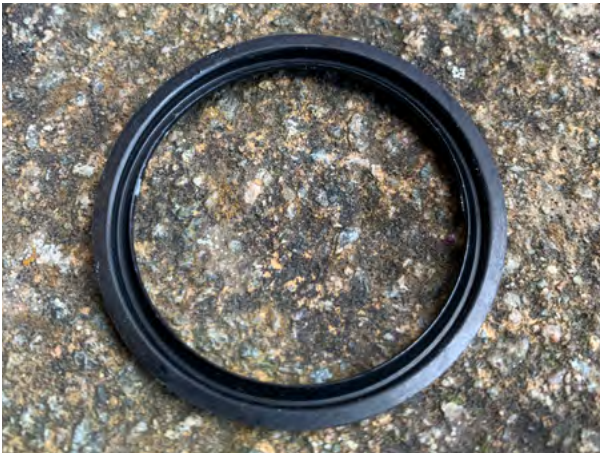
10. If you removed the hub seal in step 6, get the new seal and determine front and rear. The front of the seal has the V shape groove.
