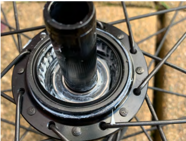
11. Push the seal into the hub shell and ensure it is correctly seated.
