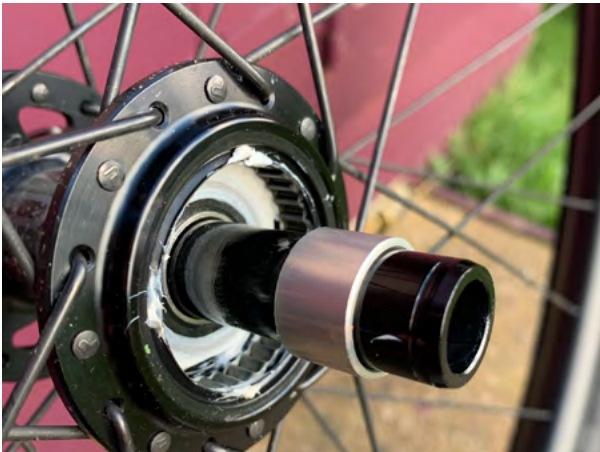
4. Remove bushing – Silver on Neutron and Black on Horizon. Note: this may be stuck in the back of the freehub.
