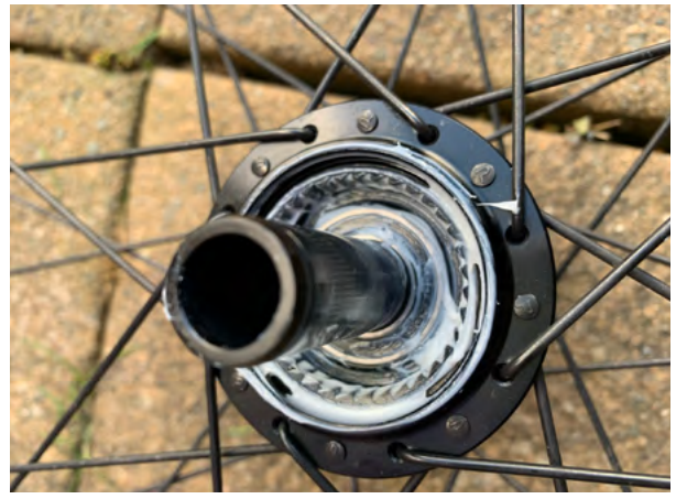
9. Apply Nukeproof hub grease to the bearing, seal seat and around the ratchet ring
