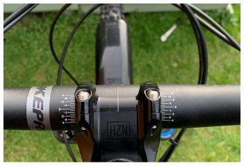
5. Straighten handlebars and tighten top cap bolt until all play has been removed from the headset. Note: You should rock the bike back and forth with the brakes on to feel for play. DO NOT over tighten bolt as this could damage the headset bearings.
