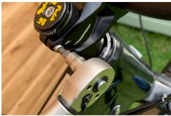
6. Tighten the stem bolts to manufacturers recommended torque setting.
