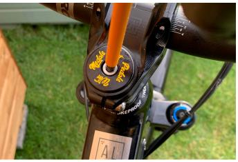
4. Start to tighten the top cap bolt.
