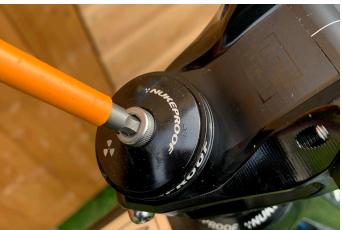
2. Loosen your top cap bolt and remove the top cap.
