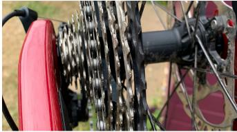
14. Cycle through the gears and check that there is no rubbing in the highest and lowest gears (you will need to do this carefully as the crankset has not been fully reinstalled). Again, washers can be added / removed to fine tune chain line if there is rubbing.
