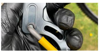
4. Using the 4mm hex key, loosen the height adjustment bolt.
