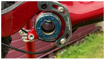
8. Rotate the back plate so it is in the 12 o'clock position and tighten ISCG bolts.
