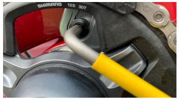
13. Tighten the height adjustment bolt. Most chain rings will allow you to do this through the gap in the ring.
