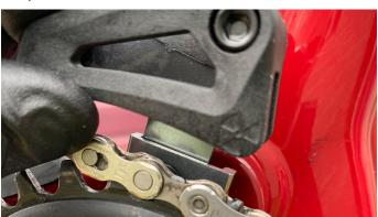
11. Lift the top guide and put the chain on the chain ring.
