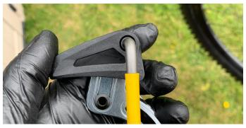
3. Using the 4mm hex key, remove the top guide from the back plate.
