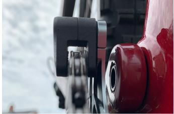
12. Lift the height adjuster to the correct height (approx. 3mm above chain) and visually check to see if the chain is in the centre of the guide. If it is, proceed to the next step. If it isn't, you will need to remove the back plate and add / remove washers as necessary to fine tune the chain line using the extra washers provided.
