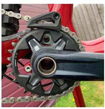
15. Now there is no rubbing and all bolts are tight the guide is setup. You can fully reinstall your crankset following the manufacturer instructions.
