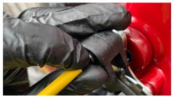
10. Reinstall the top guide using the 4mm hex key.
