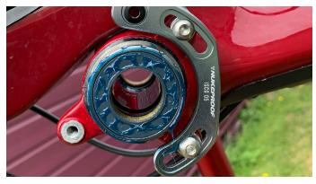
7. Use the 4mm hex key to install the back plate to the frame using the bolts and washers. The washer sits against the frame.
