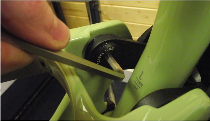
1. Remove Horse Shoe Link bolt with 6mm Allen key
