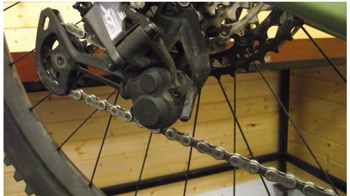
2. Put clutch into open position
