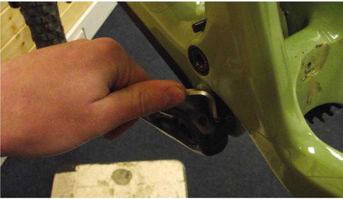
3. Loosen crank bolts with 5mm Allen Key
