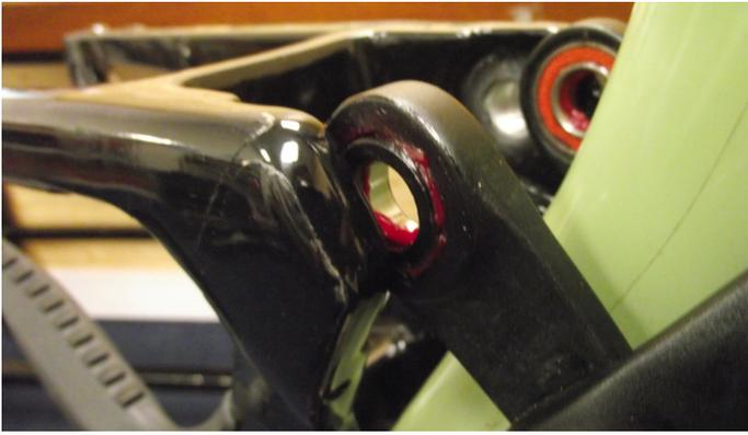
3. Place MX triangle to frame, rest on BB shell and the Horse Shoe Link will overlap at this point
