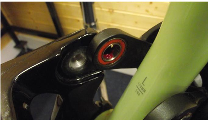
1. The MX triangle can now be installed to the Horse Shoe Link
