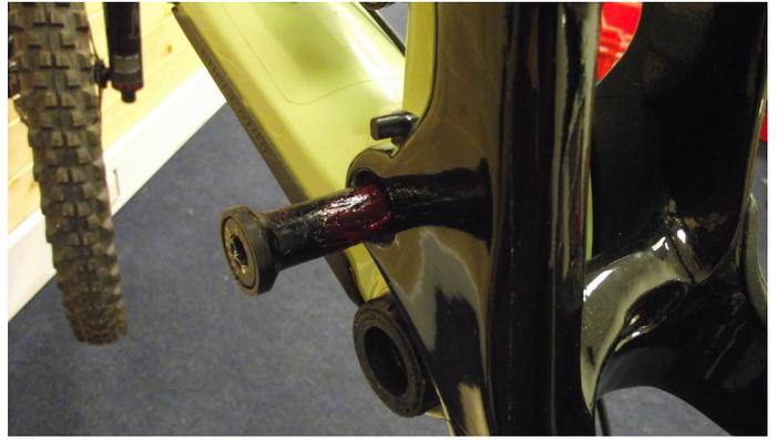
4. Install Main Pivot Bolt (25) and Collect Washer (26)
