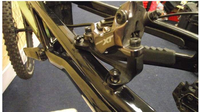
4. Place brake and thread in Brake Mount Bolts (22)
