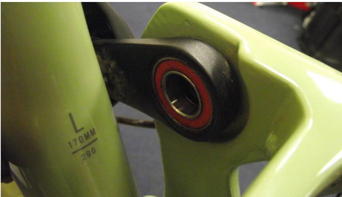
3. Bolts removed shows Bearings
