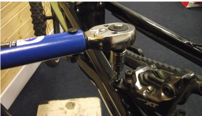
5. Tighten Brake Mount Bolts (22) to 10Nm with 4mm Allen Key Torque wrench
