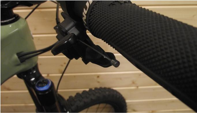
5. Remove inner gear cable
