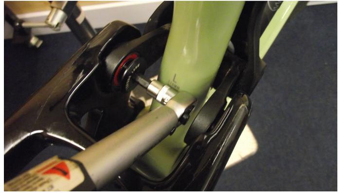
4. Tighten Horse Shoe Bolt to 19Nm with a 6mm Allen Key Torque Wrench
