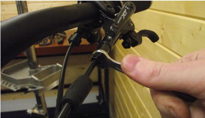
1. Remove nut cover and partially loosen nut
