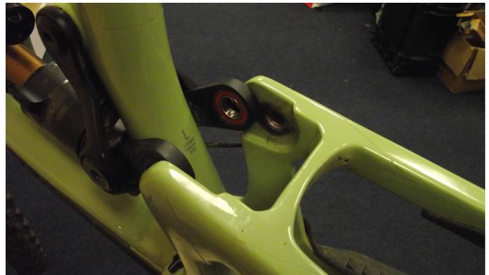
4. Allow rear triangle to rest on frames BB shell
