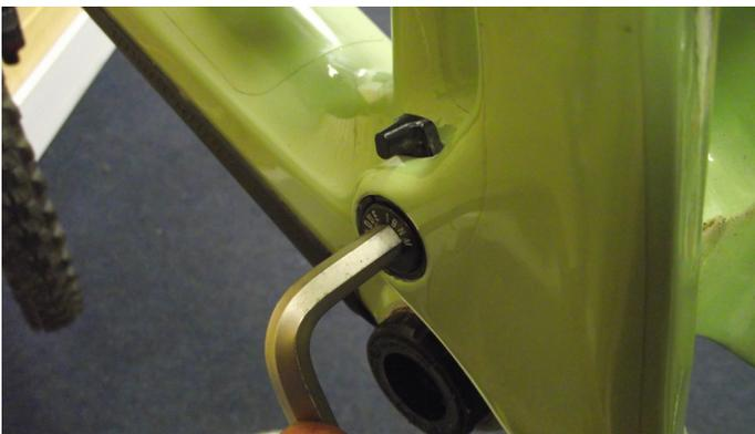
1. Undo Main Pivot bolt with 8mm Allen Key
