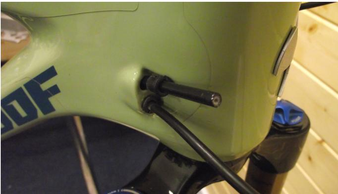
3. Hose will exit at headtube, reseal frame grommets
