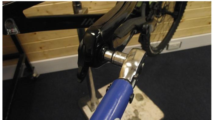
2. Install UDH and tighten to 25Nm with 8mm Torque Wrench
