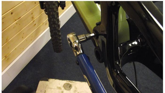
6. Tighten Main Pivot Bolt to 19Nm with 8mm Allen Key Torque Wrench
