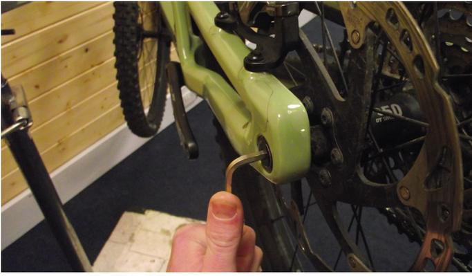
3. Remove rear axle with 5mm Allen Key
