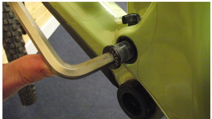
2. Remove Main Pivot Bolt (25) and Collect Washer (26)
