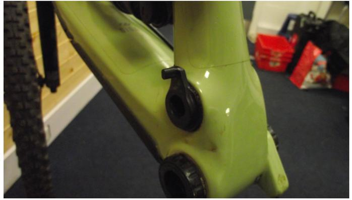
4. Main Pivot Flip Axle (24) can be left in the frame or removed for clean/grease
