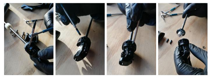
5. Undo the two grub screws to detach the actuator from the cartridge.
