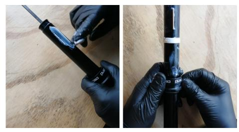
8. Grease the lower stanchion and fit the upper and lower bushing. Note the ridged bushing is the lower and the smooth is the upper.
