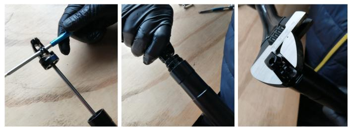
16. Push the actuator and cartridge into the base of the post and tighten with a spanner to 8Nm. You can use the shaft of a 5mm allen key through the actuator to help push it down.
