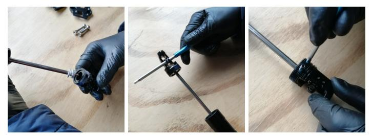
15. Fit the actuator back on to the cartridge and tighten the grub screws. Ensure the cartridge is correctly seated into the actuator. Ideally add a little Loctite 243 to the grub screws to guarantee secure fitment if there is no threadlock compound left on them.
