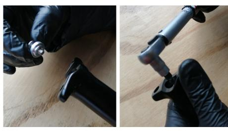
7. Insert the retaining bolt and washer into the head of the seat post stanchion and torque to 4Nm.
