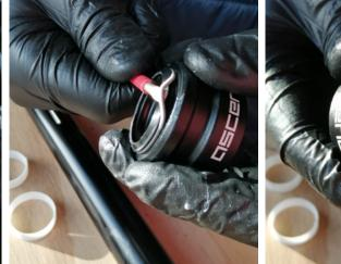
10. Disassemble the collar - remove the metal retaining ring and then lift out the rubber seal.
