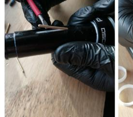
9. Using a pick or a sharp flat headed screwdriver gently lift the brass pins.
