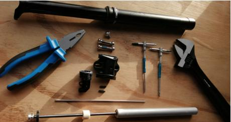
6. Remove the actuator pin from the cartridge - you should be able to pull this out with your fingers but use pliers if you can't grip it.
