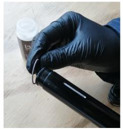
3. Slide the metal retaining ring on to the seat post stanchion.
