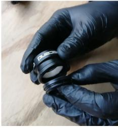
2. Insert the seal back into the collar (don't yet fit the metal retaining ring).
