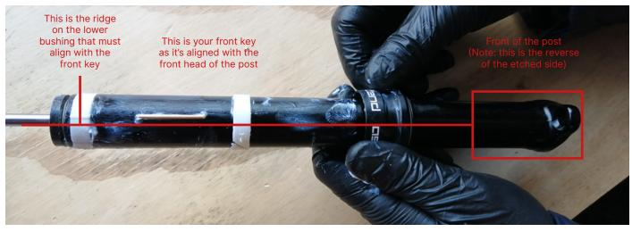
9. Grease the inserts for the keys and insert these firmly into their slots.
