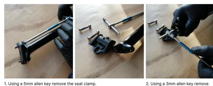
2. Using a 3mm allen key remove the top bolt and washer.
