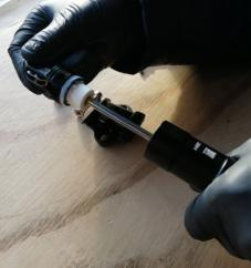
4. Remove the cartridge with the actuator still attached by pulling it out of the seatpost.
