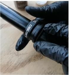
5. Push the metal retaining ring on to the seal.
