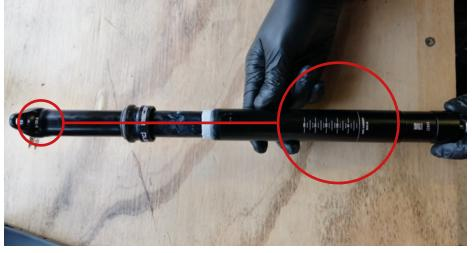
12. Insert the stanchion into the seat post tube. To guarantee alignment you can match up the laser etchings from the minimum insert markings on the seat post tube to the markings on the rear of the stanchion.
