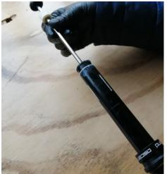
6. Insert the cartridge into the seat post stanchion.
