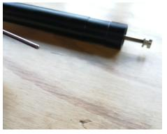
14. Insert the actuator pin into the cartridge – note the pin is directional and that the rounded end should face out of the cartridge.
