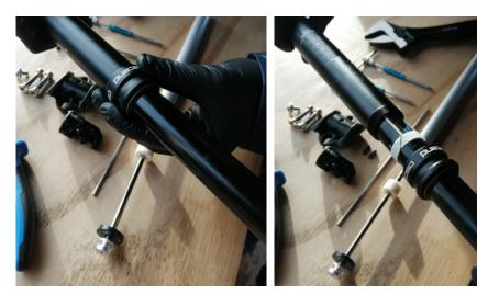
7. Unscrew the collar and remove the stanchion from the post by pulling it out.
