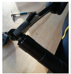
3. Using a 16mm spanner, remove the actuator head, hold the post tight and turn the actuator clockwise.
