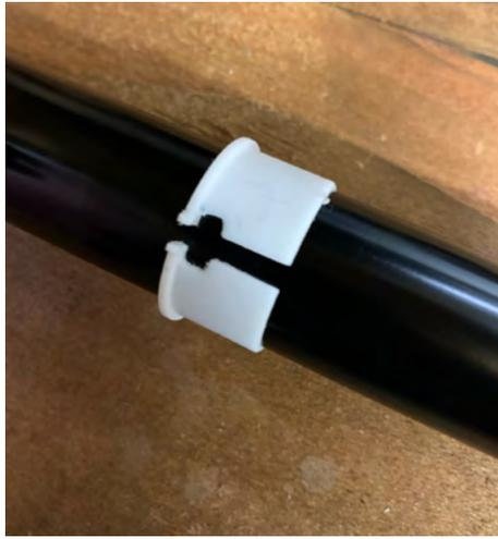
8. Get the larger bushing and slide it onto the stanchion. It should go on with the lip to the top.
