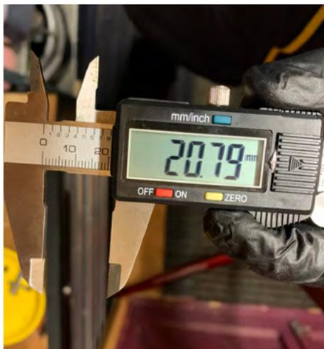
29. Measure the height from bottom of actuator to top of mechanism using Vernier callipers. Adjust cable so that the height between 20.5mm – 21.5mm.
