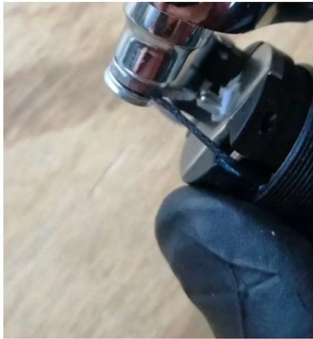
2. Using a 8mm socket carefully undo the nut to release the nylon thread.
