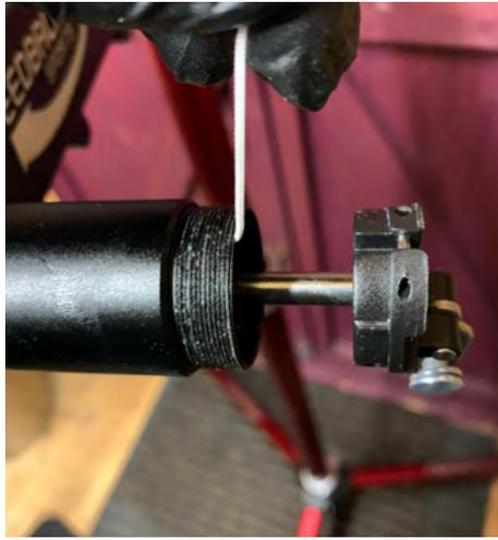
25. Lift the string into the slot inside the post and then push the cartridge / actuator into place. Note that the slot in the actuator needs to go in line with the string.
