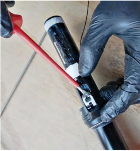
11. Remove the actuator nylon thread and the metal housing.
