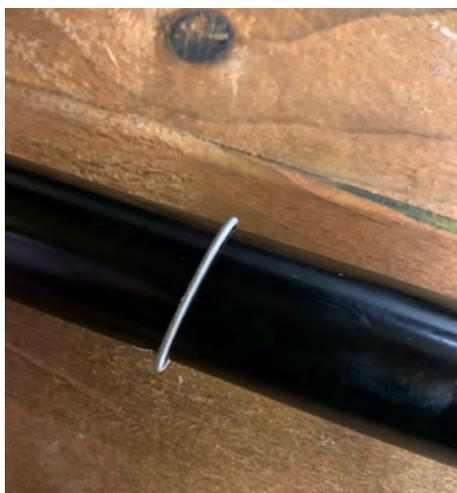
5. Get the metal retaining ring from the seal and slide this onto the stanchion.
