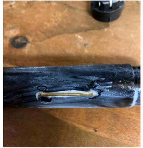
9. Apply grease to the bottom half of the stanchion and then reinsert brass keys.
