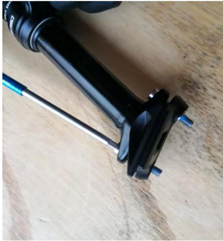
5. Remove the actuator pin from the cartridge - you should be able to pull this out with your fingers.
