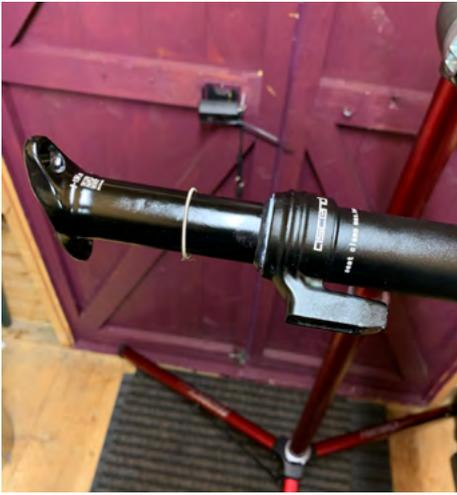
18. With the stanchion now in place, slide the bushing down into place and then slide the collar down into place.
