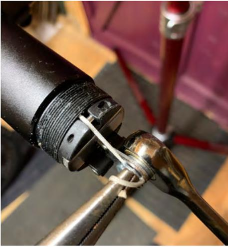
30. Tighten the nut using an 8mm spanner or socket.
