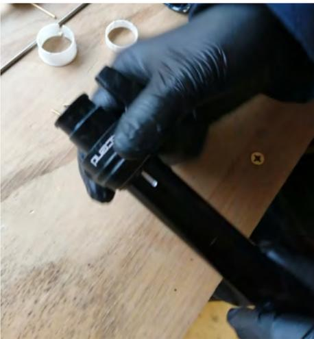
15. Remove the collar and disassemble - carefully removing the retaining ring, inner seal and O-ring.
