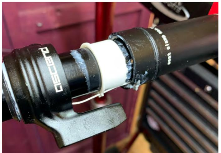
17. Carefully insert the stanchion into the post, if everything has been lined up correctly in the steps above it should slide in easily. If you feel resistance, STOP and repeat step 13 onwards. Failure to stop will result in the string being damaged.
