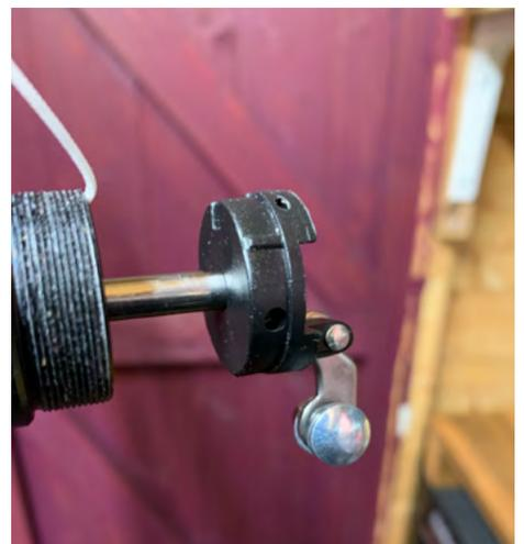
23. Get your actuator and push it onto the bottom of the cartridge. The bolt hole in the actuator should line up with the indent in the cartridge.
