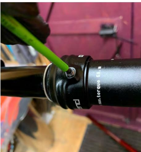
21. Replace the bolt on the collar to hold it in place.
