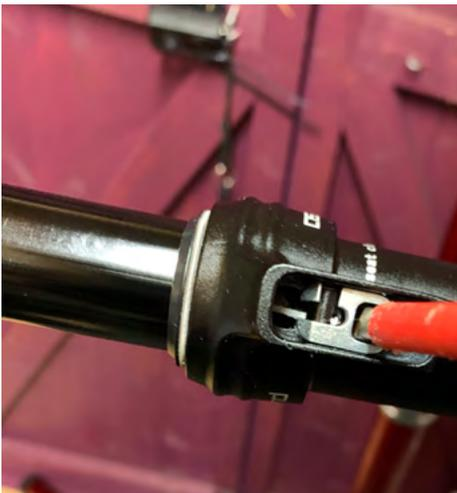
33. You can now push the actuator carefully using a flat head screwdriver to activate it. The post should extend. You can push the actuator again and push the post to ensure it functions as it should. If the post is not working as expected, compress halfway, remove the bottom cap and repeat from step 29 onwards.
