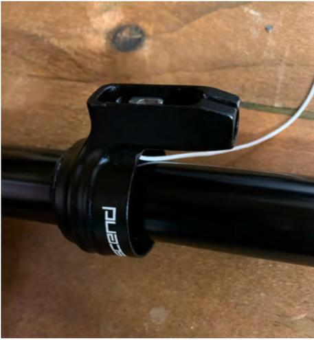
7. Slide the collar onto the stanchion, double check the seal is positioned correctly and is not folded over.
