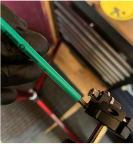
24. Replace the bolt to hold the actuator in place. Be careful not to overtighten. The bolt should not be visible from the opposite side of the actuator.
