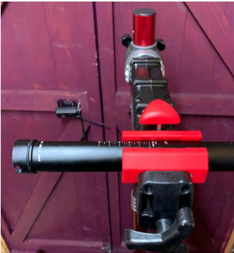
10. Take the bottom part of the seatpost and clamp it horizontally in a workstand with the rear of the post (laser etched markings) facing upwards.
