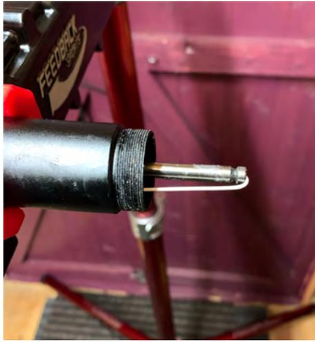
19. Carefully push the stanchion down so the bottom of the cartridge is visible.
