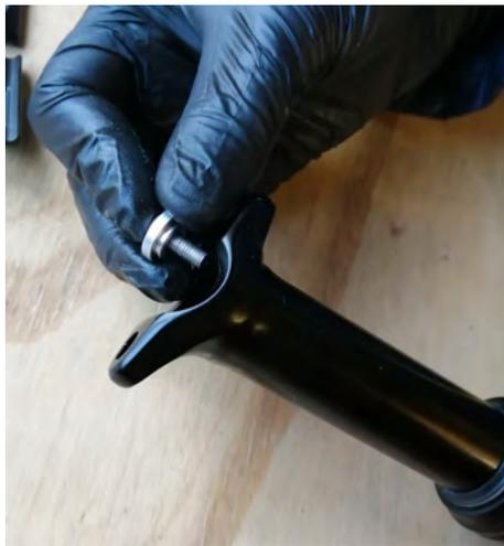
7. Using a 3mm allen key remove the bolt and washer from the head assembly.
