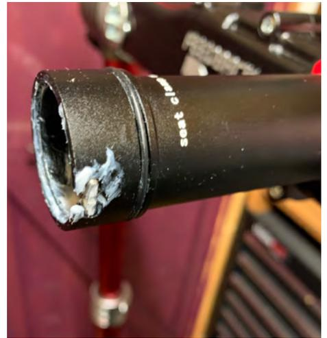
12. Grease cable guide and inner part of post.
