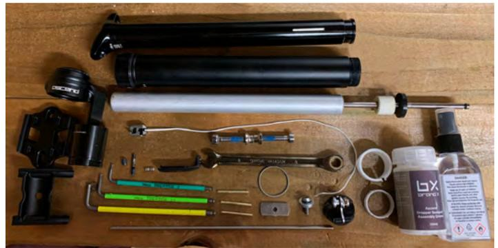
Note – Before you start, **ensure that your cartridge has been compressed halfway**. You can do this by inserting the pin and then pushing down on the cartridge.
