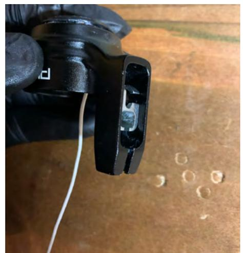
6. Get the string, insert the barrel into the metal piece with the rounded side facing outwards then feed string through the hole in the collar.
