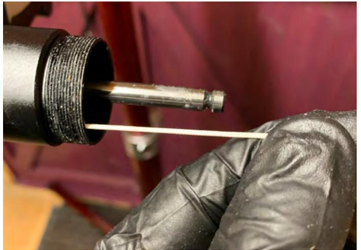
20. Gently pull the string and ensure it moves freely and moves the actuator up, then push the actuator down with your finger to ensure it pulls the string – repeat this step a few times to ensure that the string is moving with no resistance. If the string does not move freely, you will need to remove the stanchion from the post and start from step 13 to reinstall correctly.
