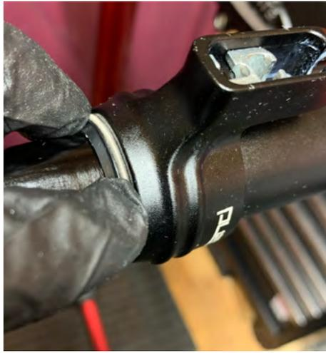
31. Refit the metal retaining ring on the seal.
