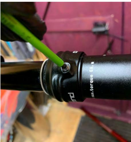
28. Take the bolt and washer, insert the string through the hole, push the bolt into the actuator then fit washer and nut.
