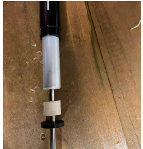
3. Get your cartridge, find the thicker end with the threaded hole and push inside the stanchion then fit the foam spacer and rubber dampner.
