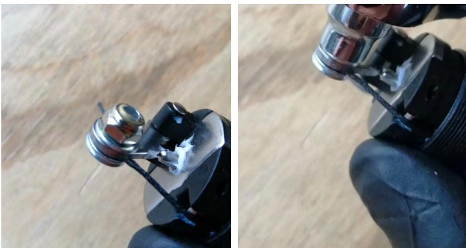
2. Using a 8mm socket carefully undo the nut to release the nylon thread.
