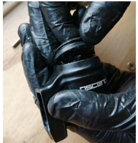
15. Remove the collar and disassemble - carefully removing the retaining ring, inner seal and O-ring.
