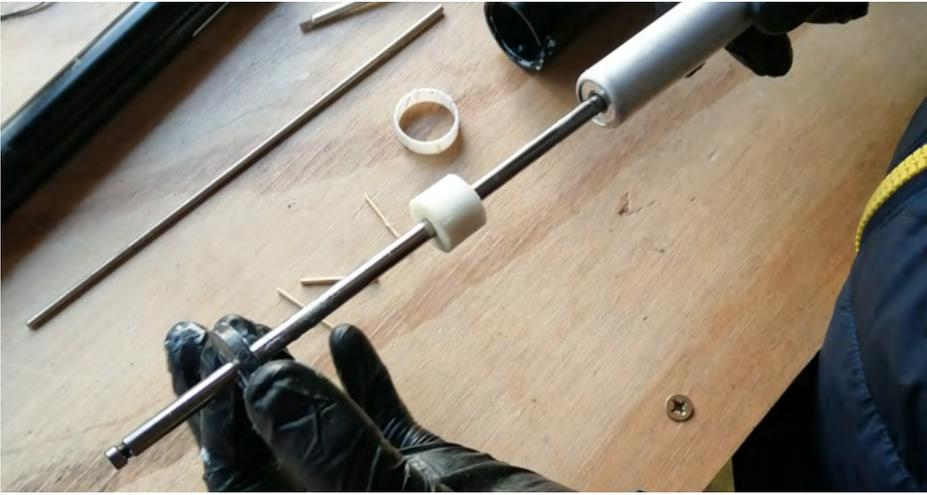
16. Remove the rubber dampener and foam spacer from the cartridge.
