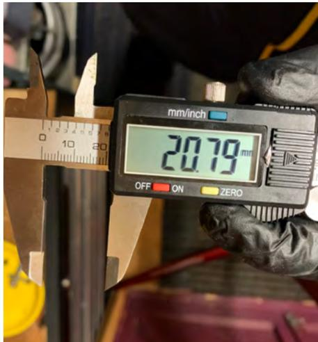
29. Measure the height from bottom of actuator to top of mechanism using Vernier callipers. Adjust cable so that the height between 20.5mm – 21.5mm.
