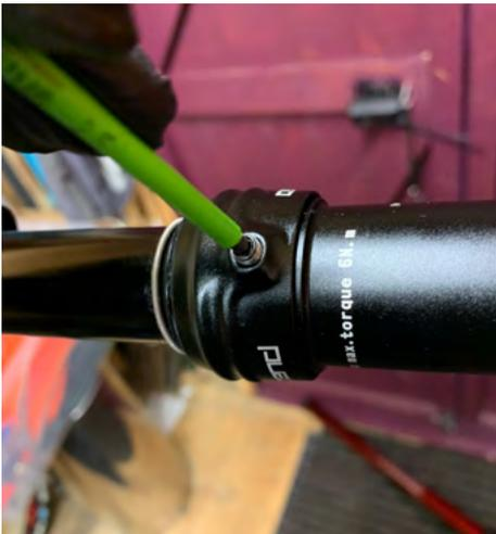
28. Take the bolt and washer, insert the string through the hole, push the bolt into the actuator then fit washer and nut.
