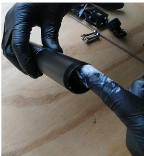
11. Lubricate the inner of the seat post tube.
