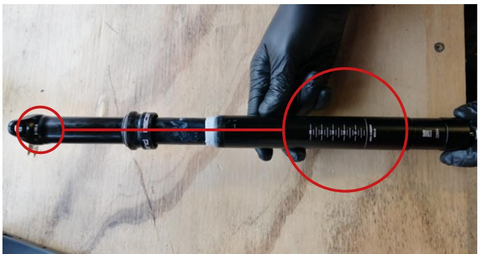
12. Insert the stanchion into the seat post tube. To guarantee alignment you can match up the laser etchings from the minimum insert markings on the seat post tube to the markings on the rear of the stanchion.
