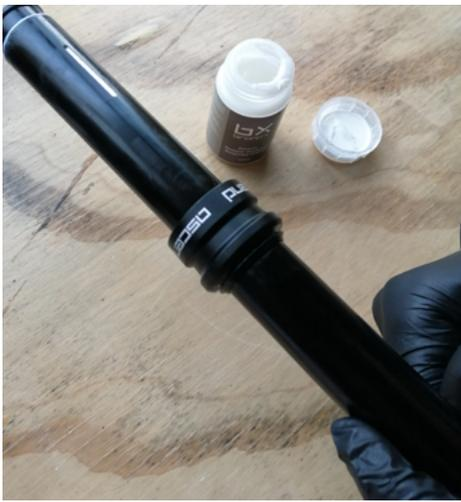
4. Feed the collar on to the seat post stanchion - check the seal has not curled over and is uniform and in place on the collar.
