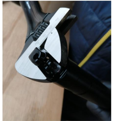
16. Push the actuator and cartridge into the base of the post and tighten with a spanner to 8Nm. You can use the shaft of a 5mm allen key through the actuator to help push it down.
