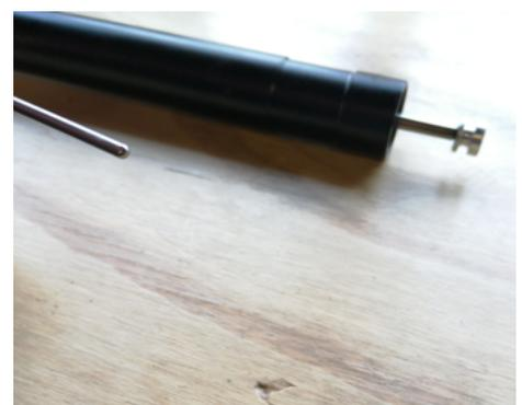
14. Insert the actuator pin into the cartridge – note the pin is directional and that the rounded end should face out of the cartridge.
