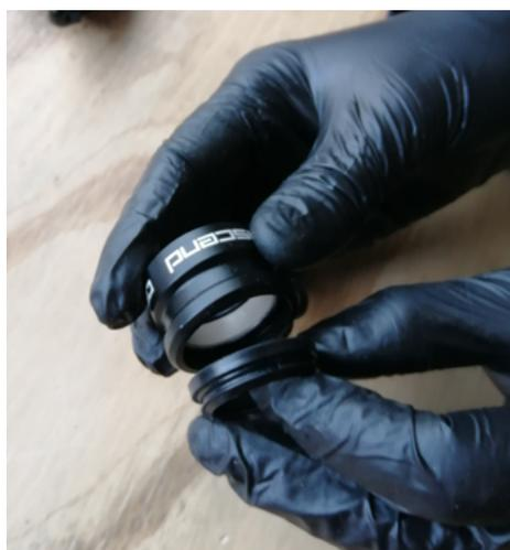
2. Insert the seal back into the collar (don't yet fit the metal retaining ring).
