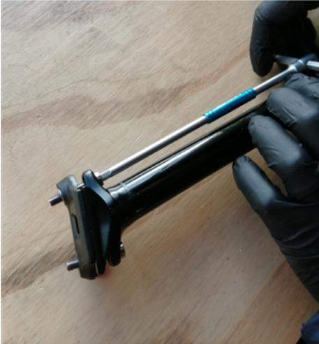
1. Using a 5mm allen key remove the seat clamp.
