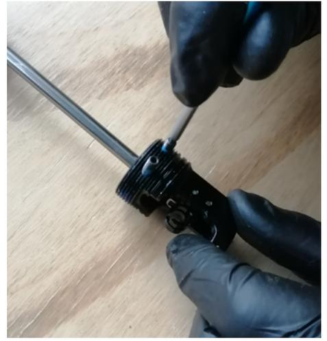
15. Fit the actuator back on to the cartridge and tighten the grub screws. Ensure the cartridge is correctly seated into the actuator. Ideally add a little Loctite 243 to the grub screws to guarantee secure fitment if there is no threadlock compound left on them.
