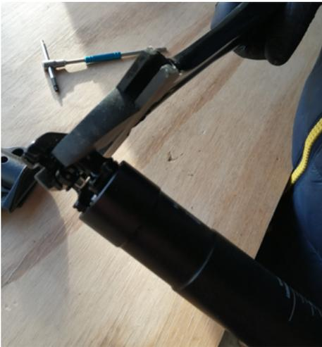
3. Using a 16mm spanner, remove the actuator head, hold the post tight and turn the actuator clockwise.
