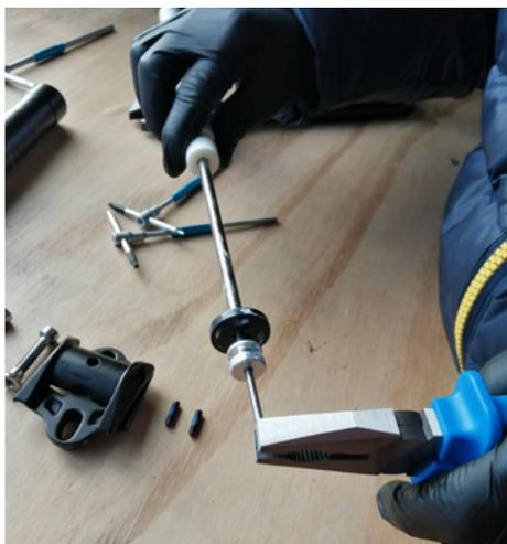
6. Remove the actuator pin from the cartridge - you should be able to pull this out with your fingers but use pliers if you can't grip it.
