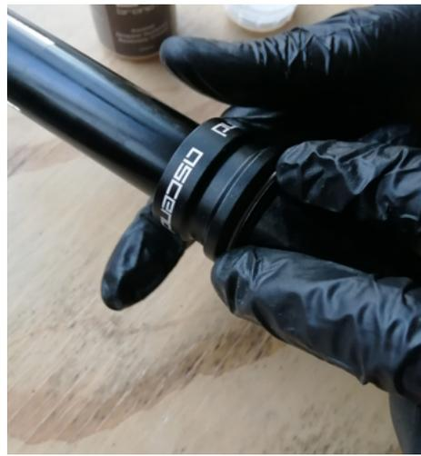
5. Push the metal retaining ring on to the seal.
