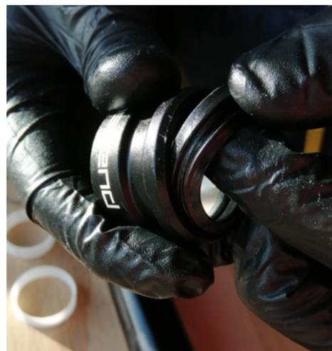
10. Disassemble the collar - remove the metal retaining ring and then lift out the rubber seal.
