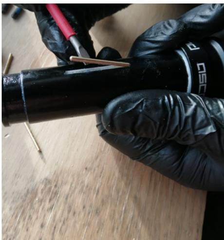
9. Using a pick or a sharp flat headed screwdriver gently lift the brass pins.
