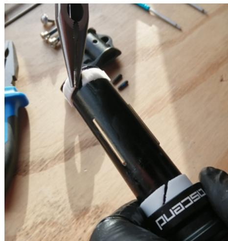
8. Delicately remove the upper and lower bushing and collar. Note the orientation of the lower bushing. This is important for reassembly.
