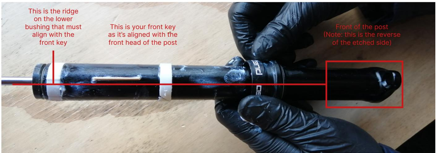
9. Grease the inserts for the keys and insert these firmly into their slots.
