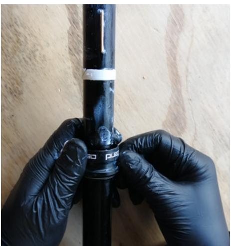
8. Grease the lower stanchion and fit the upper and lower bushing. Note the ridged bushing is the lower and the smooth is the upper.
