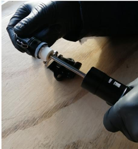
4. Remove the cartridge with the actuator still attached by pulling it out of the seatpost.
