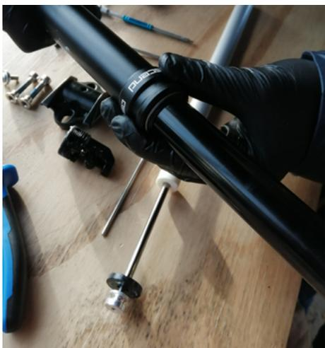
7. Unscrew the collar and remove the stanchion from the post by pulling it out.
