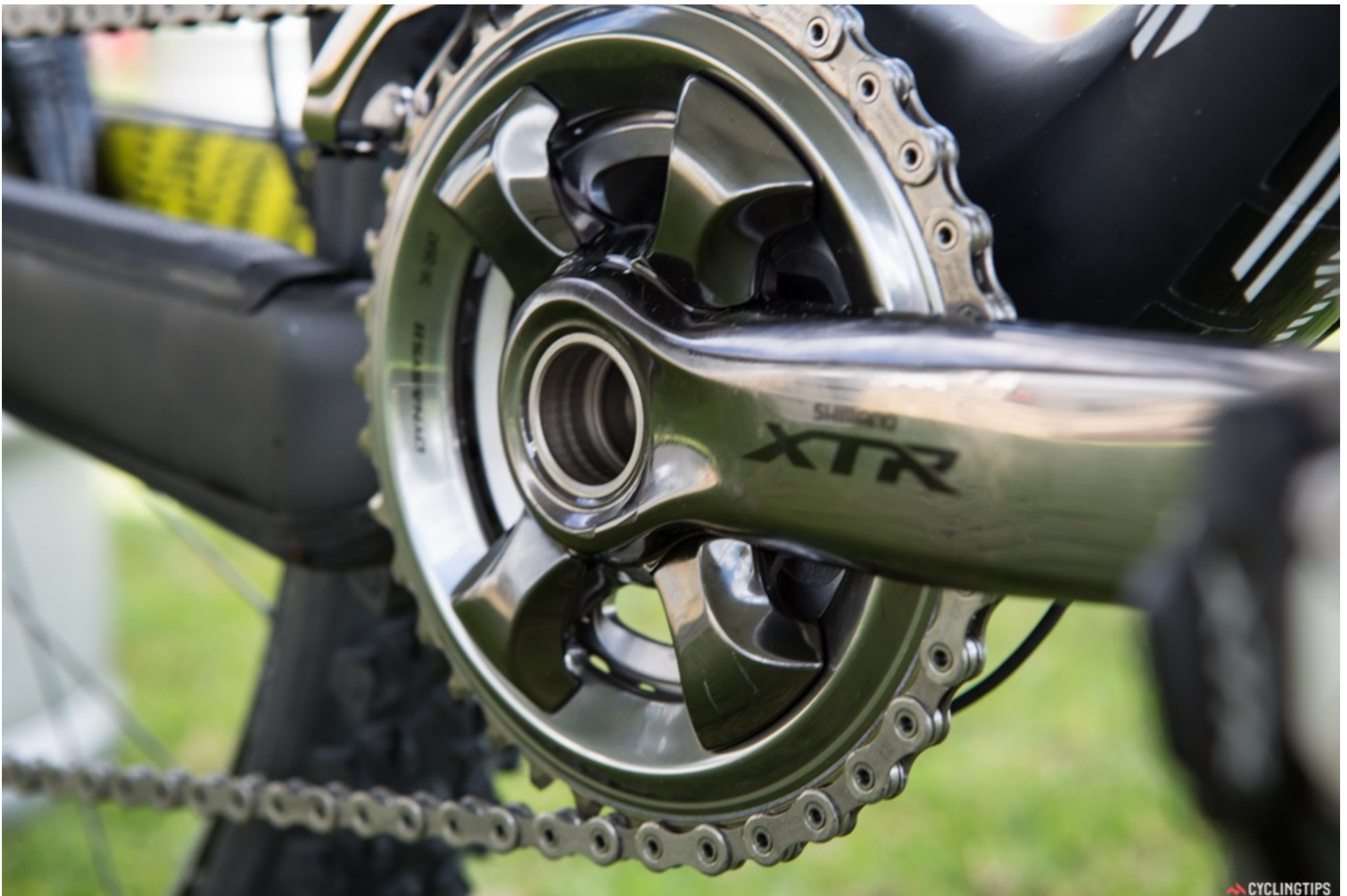
XTR M9050 cranks are a mix of aluminium, carbon and alloy and employ Shimano's Hollowtech design
