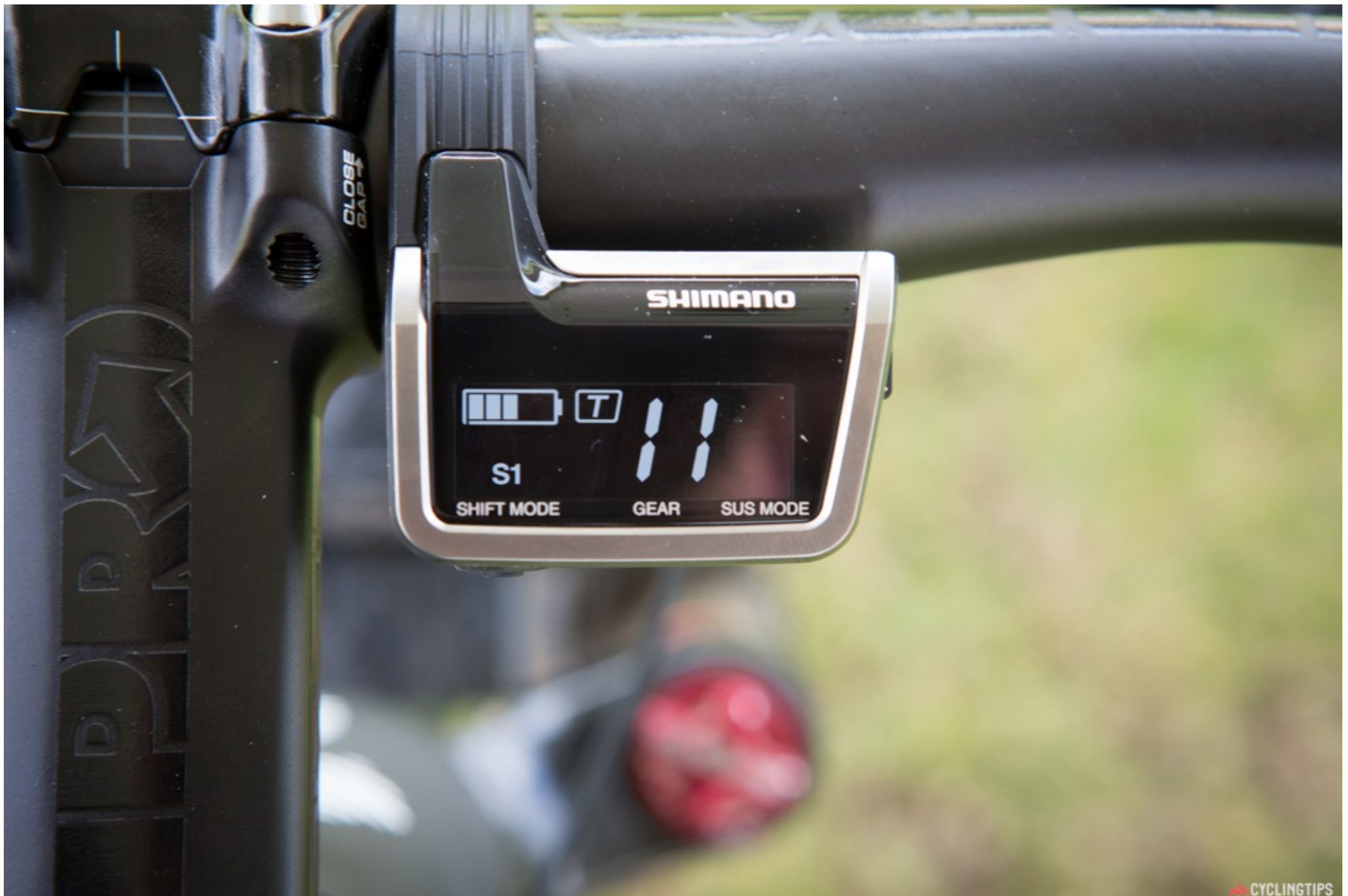
The shifting indicator shows the battery life so you won't forget about it. During 80km of riding, the
