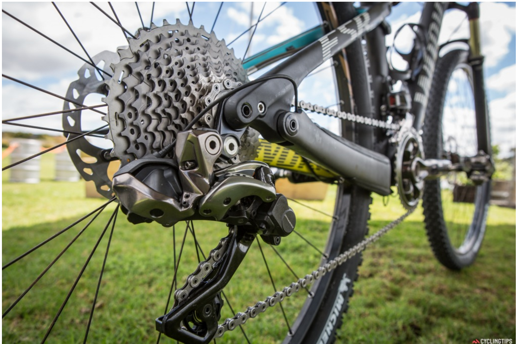
The new XTR M9050 cassette is built with a carbon spider, aluminium, titanium and steel cogs mix, and
