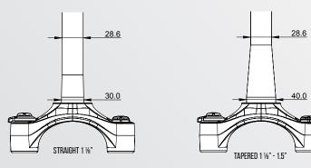
Measure the internal diameter of the head tube for both the top & bottom sections (after you have removed the headset cups from the frame).
