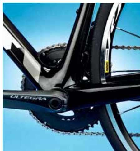
An oversized down tube, flared seat tube and BB386EVO bottom bracket (above) provide a stiff platform for efficient power transfer; Ultegra brakes (right) are easily metered and reliable
