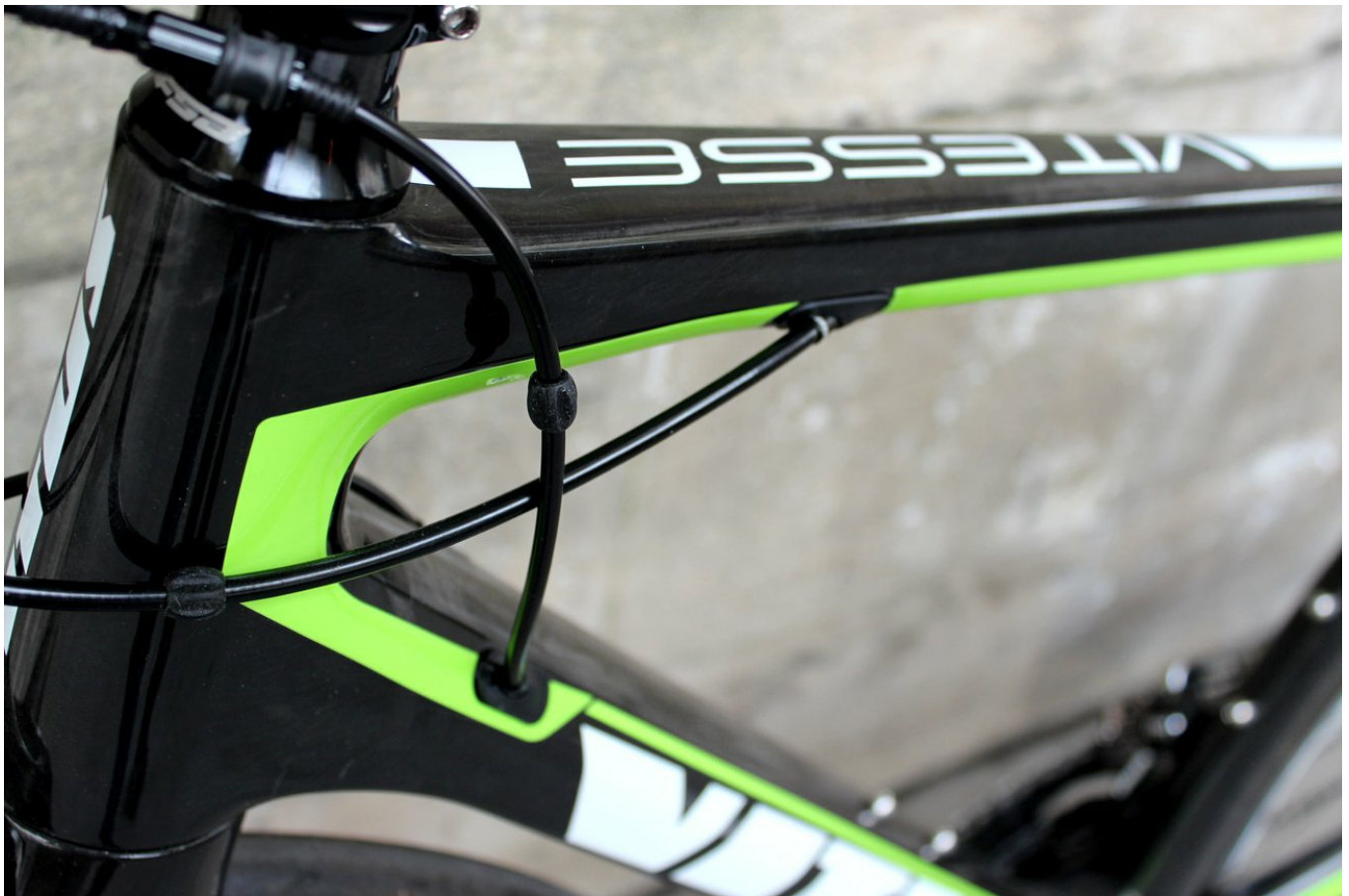
📷 Internal cable routing keeps things neat and tidy
