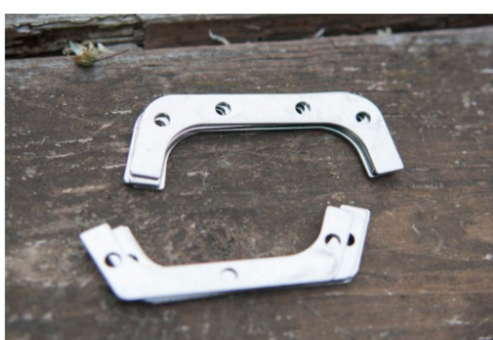
pb Steel shims can be used to customize the platform height to suit different shoes and rider preferences.
