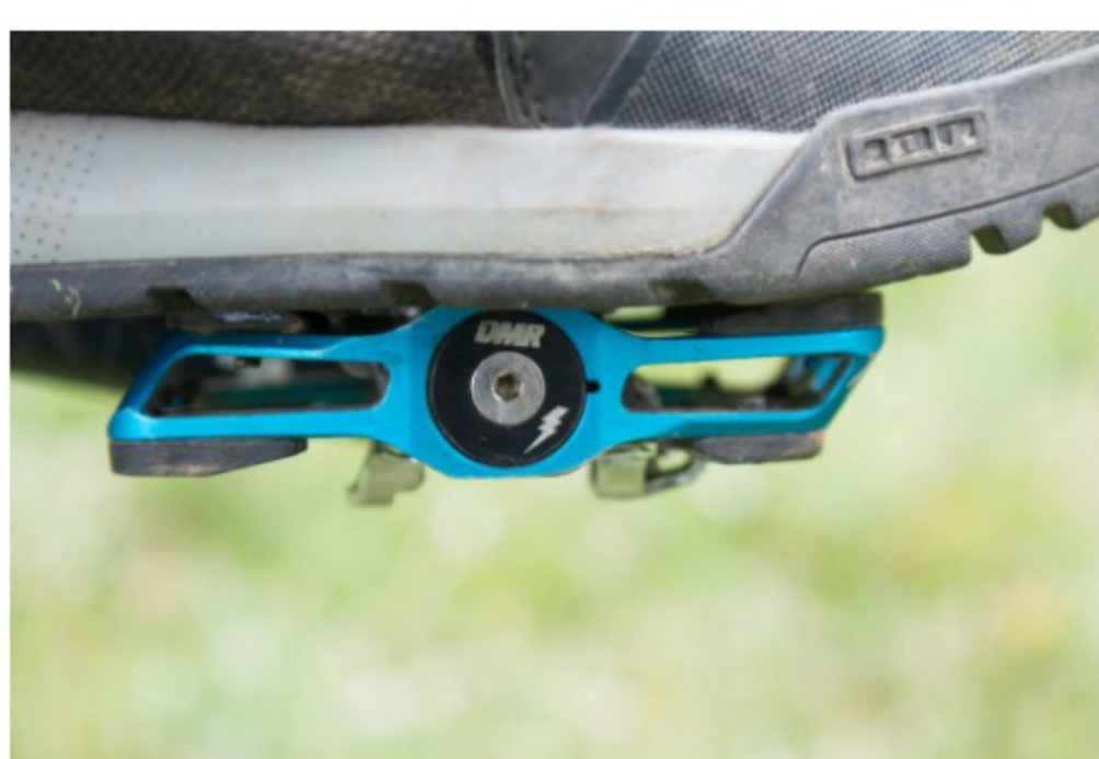
pb Steel shims can be used to customize the platform height to suit different shoes and rider preferences.
